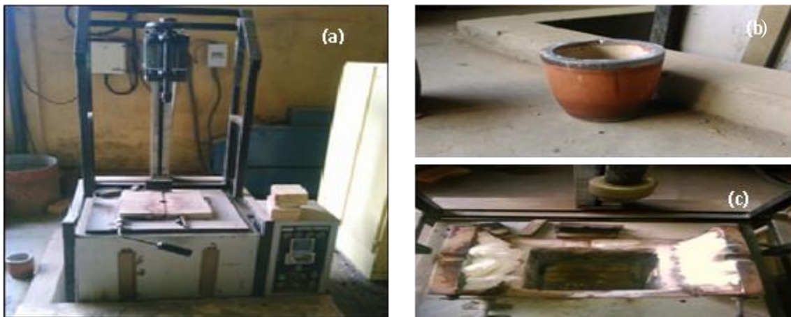
Figure 3.2: Stir casting setup (a) Furnace with motor and temperature controller (b) Graphite crucible, (c) Muffle furnace [Photo Courtesy: Central Workshop at Thapar University]
