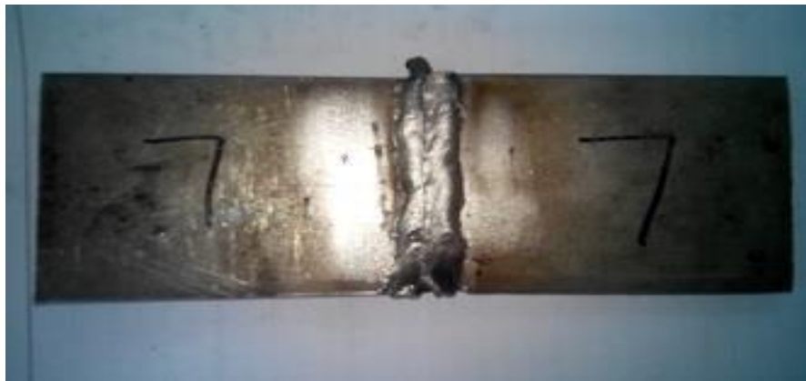
Figure 3.7: Plates after three passes of welding.
