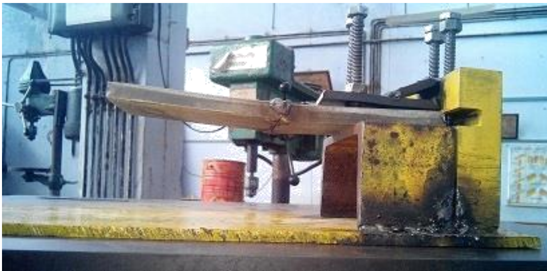
Figure 3.18: Distortion measurement setup.
