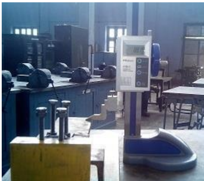
Figure 3.19: Height gauge used for measuring height.
