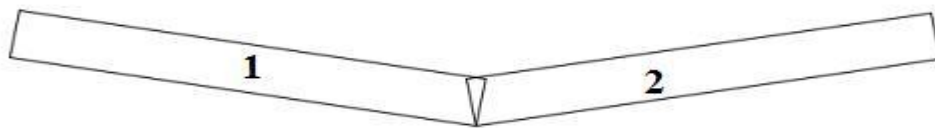
Figure 3.16: Distorted plates after welding
