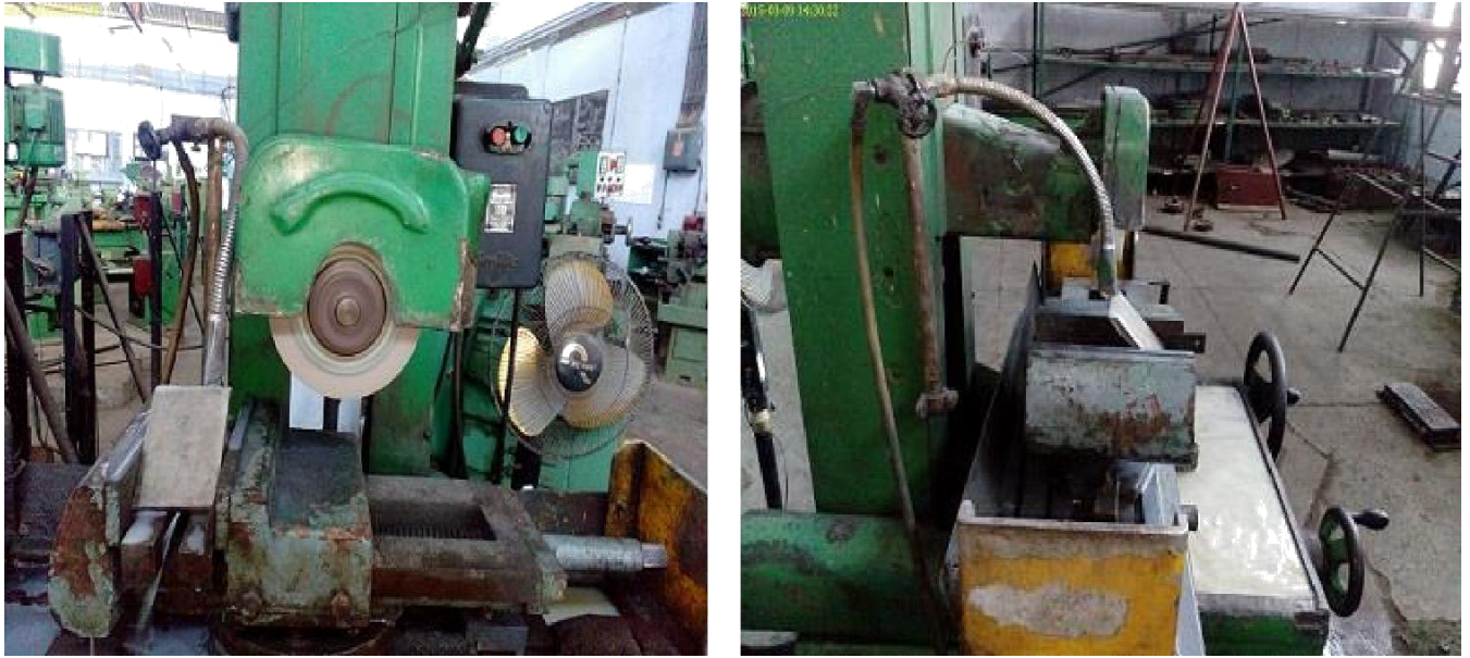
Figure 3.4: Edge preparation of plates on surface grinding machine.
