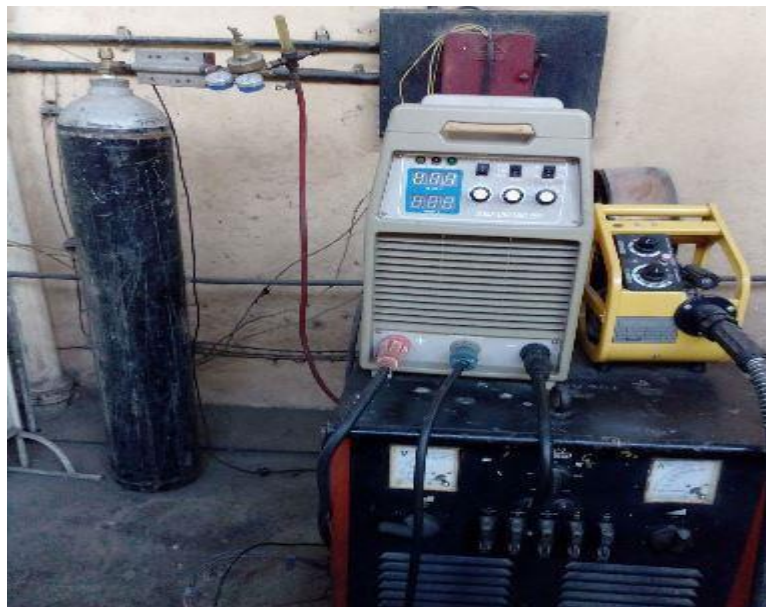
Figure 3.1: Set up of semi-automatic MIG machine (Courtesy: Central Workshop, Thapar University, Patiala)
