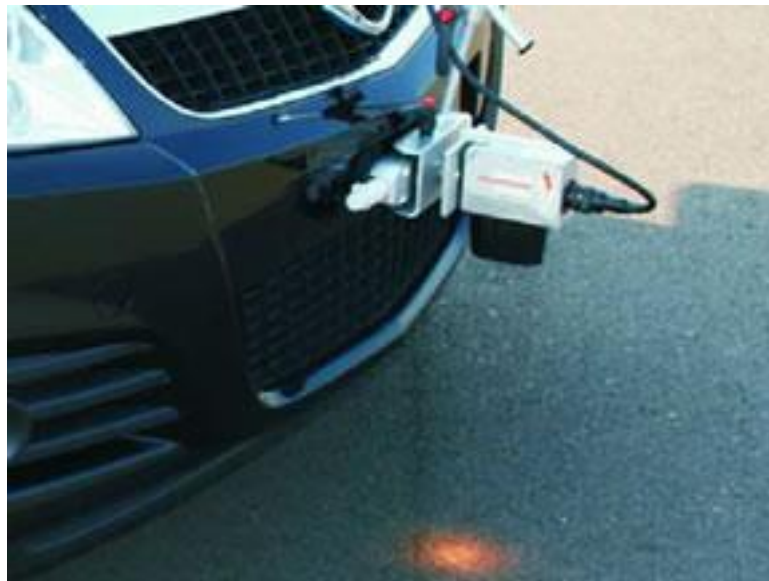
Fig. 3.3. Speed Sensor Mounting Position
