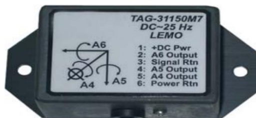
Fig. 3.9. Gyro Sensor used to capture roll rate and pitch rate of test vehicle
