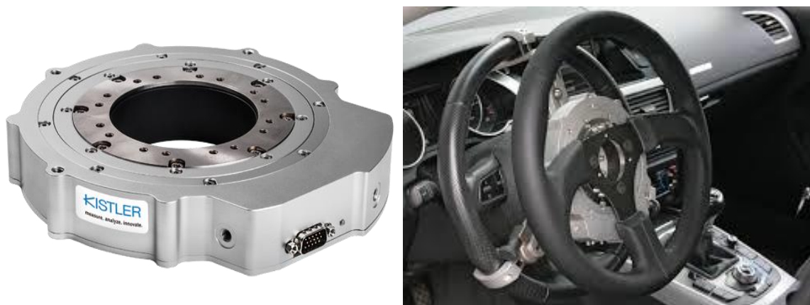
Fig. 3.4. MSW Sensor & Mounting Position
