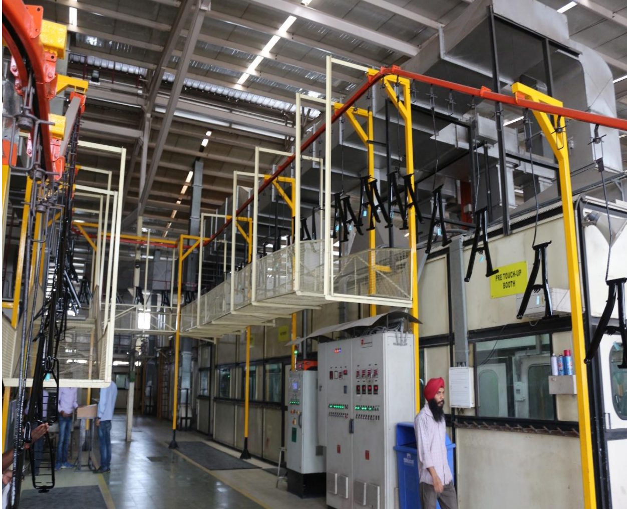
Figure 4.2.2: Electrostatic Disk type Paint Shop
