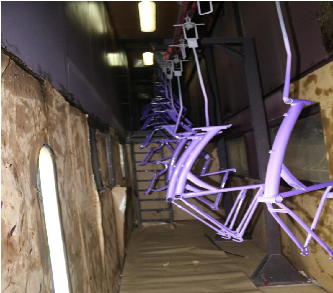
Figure 4.2.4: Bicycle parts going into the heat exchanger chamber through conveyor
