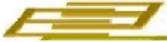
Fig. 6.9 IDT structure for detection of resistance change of sensing surface
