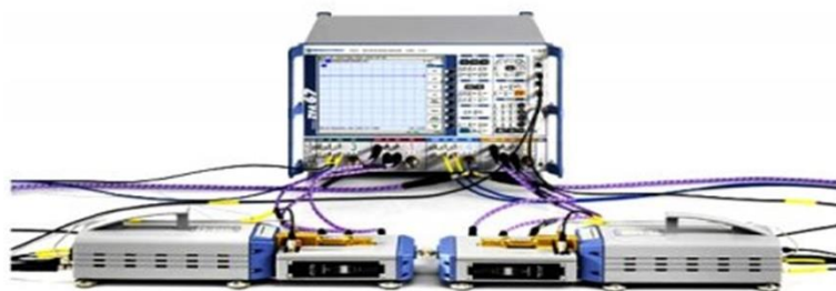
Figure 3.18: Experimental setup for electromagnetic shielding effectiveness measurement.
