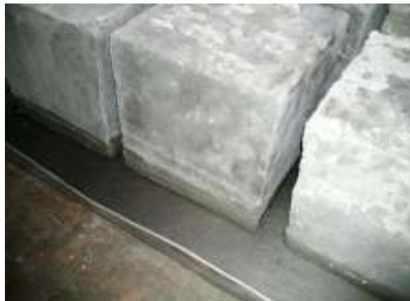
Fig.4.18:- Specimen immersed and Sealed with water seal.
