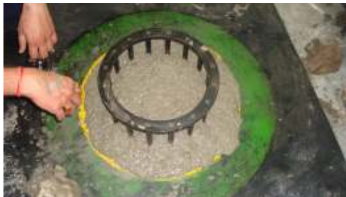
Fig. 4.14: Slump Flow test –SCC-100%RFA
