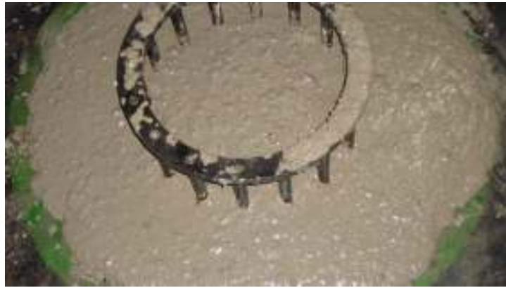
Fig. 4.13: Slump Flow test –SCC-C
