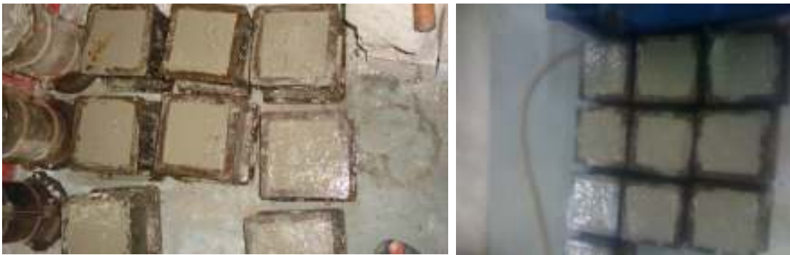
Fig 4.9 Specimen Curing (Recycled & Fresh)
