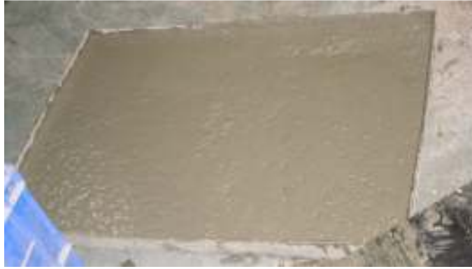
Fig 4.7 SCC made with Fresh Aggregate
