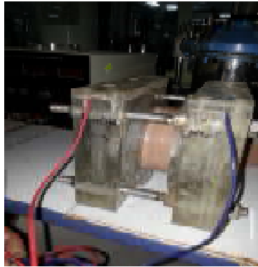
Fig 4.20: - Typical Cell Arrangement with Reservoir(RCPT)
