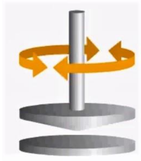
Figure 3.13 Movement of Oscillation Test in DSR
