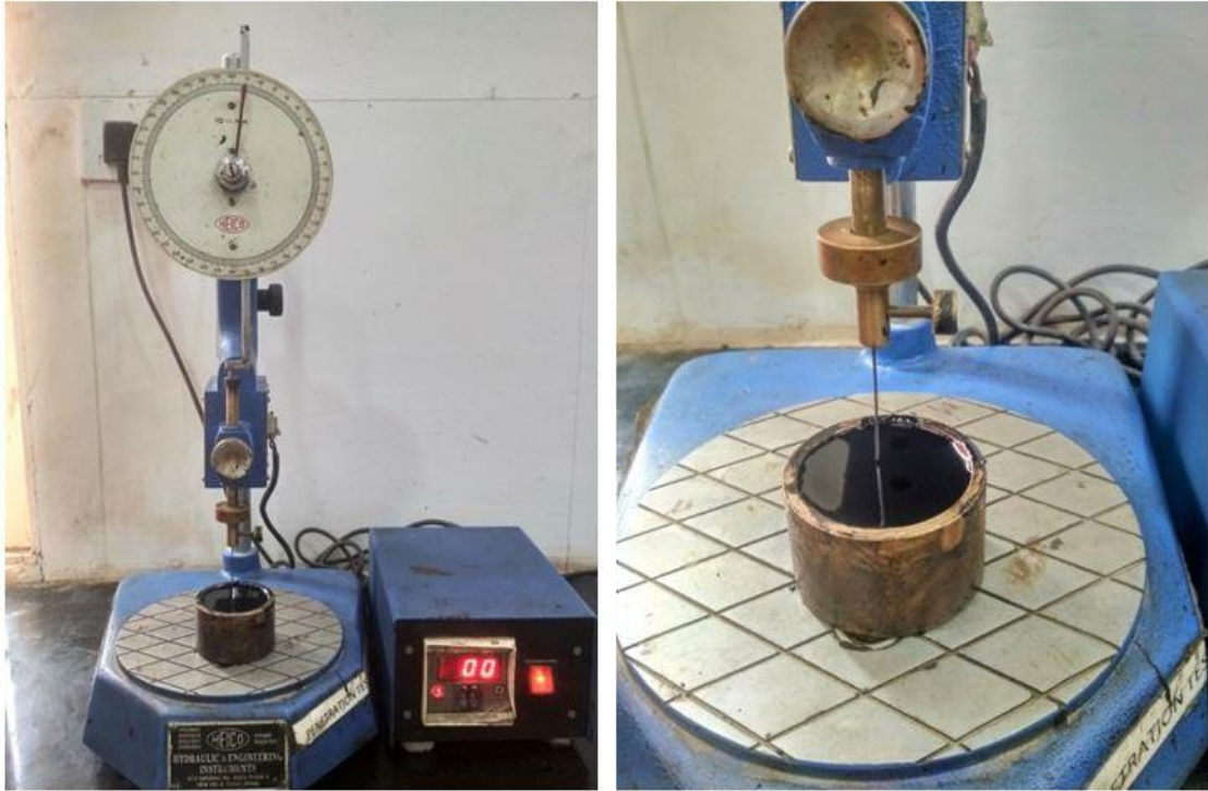
Figure 3.6 Penetrometer Instrument with Sample
