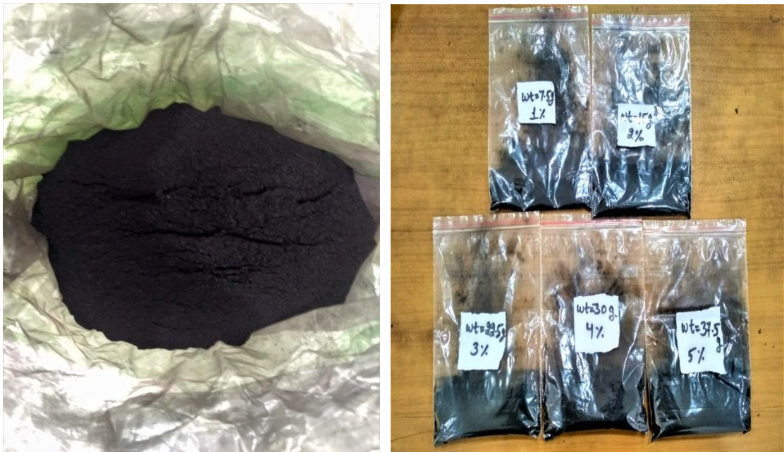
Figure 3.2 Coconut Shell Micro Charcoal Powder
