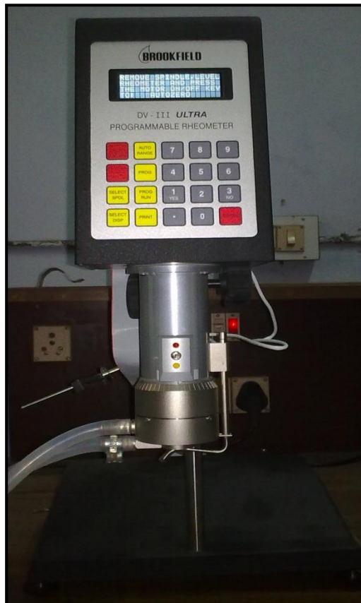
Figure 3.5 Cone and plate type Brookfield LVDV-III-Pro viscometer
