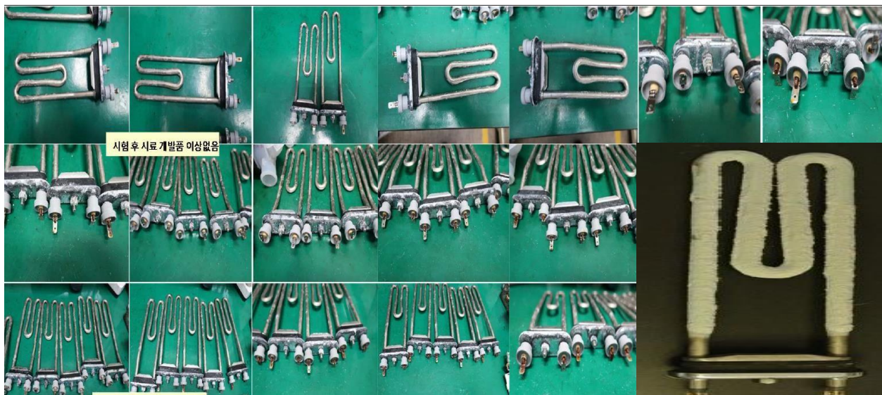
Fig.(e) Dismantled heater part of the HEDD washing machine with limestone accumulation
