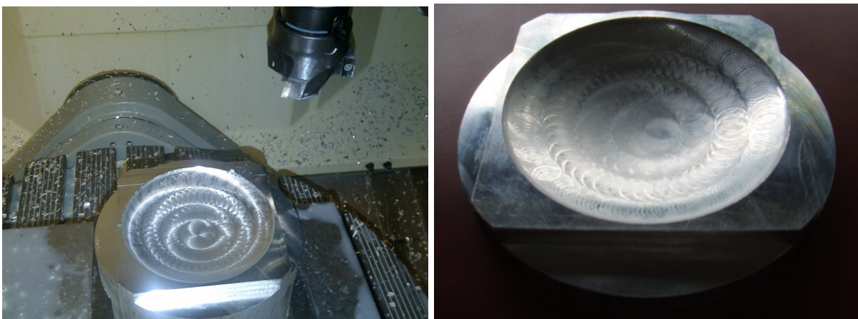
Figure 5.15: 5-axis machining results for spherical test part [65]
