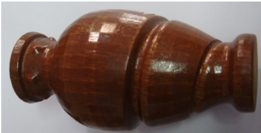
Figure 1.9: Flat facets appearing on the STL part machined using a ball-nosed end mill.
