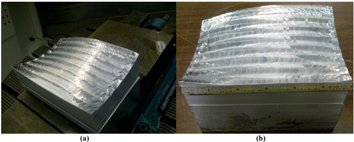
Figure 5.18: Results of 5-axis machining of the bi-quadratic Bezier test part [65]
