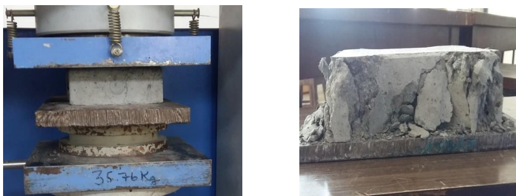
(a) Cracks during testing
