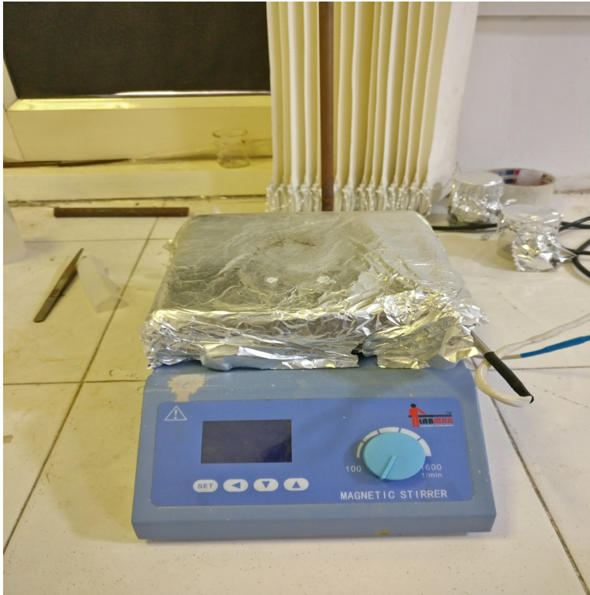
Figure 6.3 Hot plate used for soft baking
