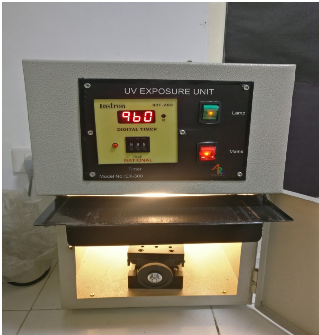
Figure 6.4 UV exposure unit used for exposing the sample to UV light
