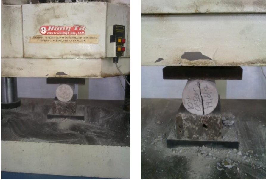
Fig. 3.13: Universal testing machine (UTM) for split tensile strength testing of concrete
