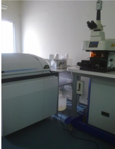
Fig. 3.16: Inductively coupled plasma mass spectrometry (ICP-MS) instrument for metal analysis
