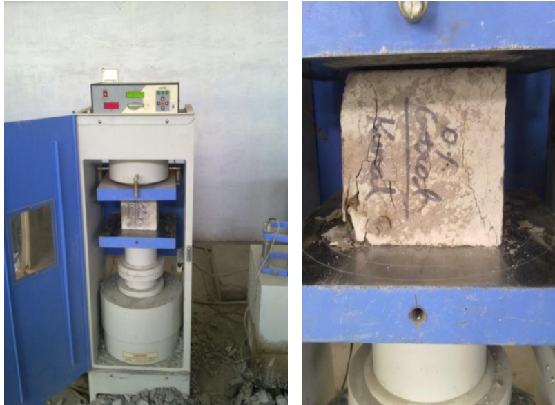
Fig. 3.12: Compression testing machine (CTM) for compressive strength testing of concrete
