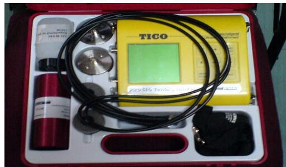
Fig. 3.14: Ultrasonic pulse velocity apparatus (TICO instruments)
