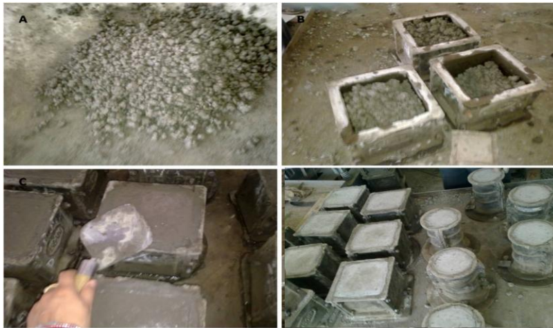
Fig 3.11: Casting of concrete cubes and cylinders (M20)
