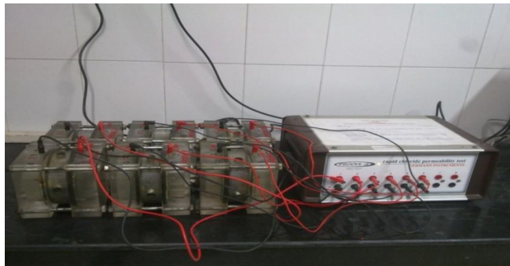
Fig. 3.15: Set up of rapid chloride permeability test (PROOVE'it, Germann Instruments)
