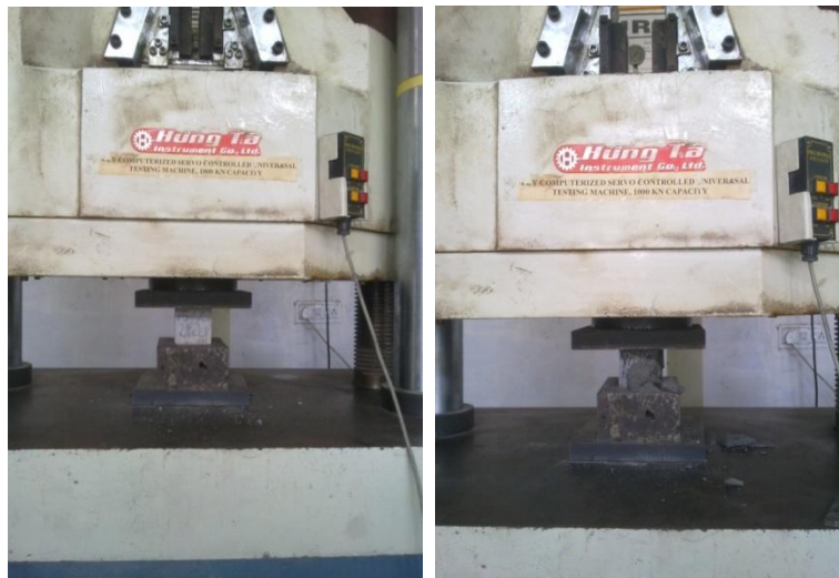
Fig. 3.10: Universal testing machine (UTM) for compressive strength testing of mortar
