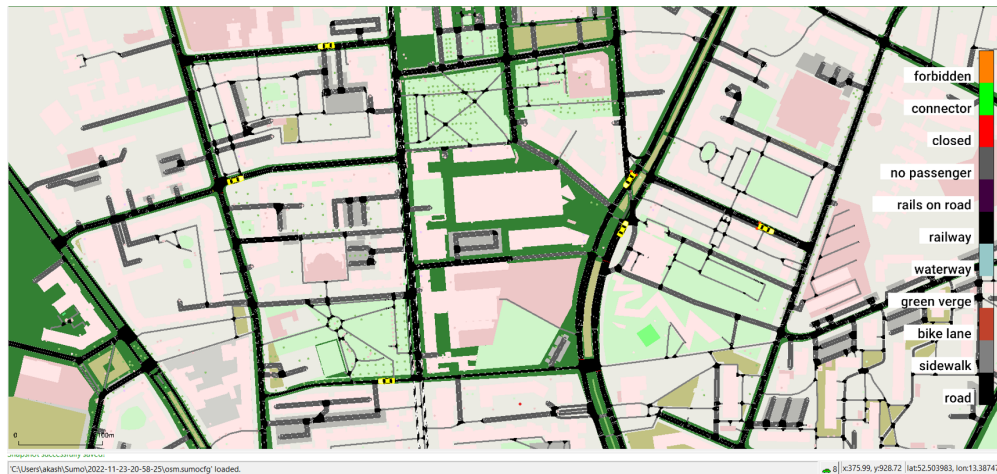
Figure 4.3: Area selected for network traffic simulation in SUMO
