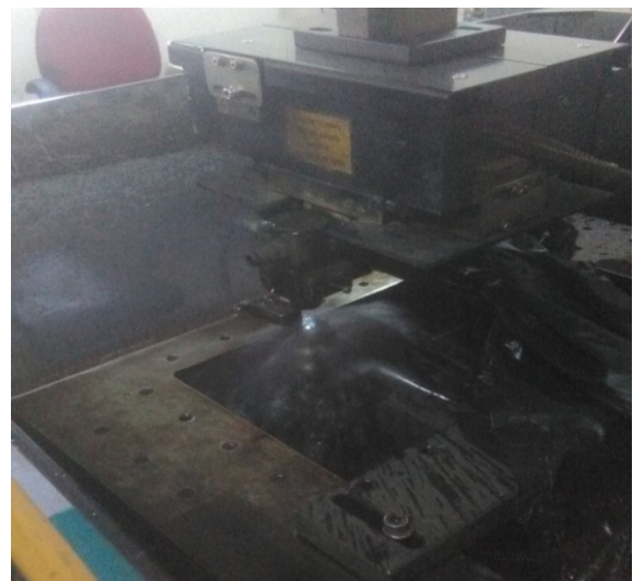
Fig. 3.9 (a) Wire feed mechanism with spool of wire and (b) operations in progress
