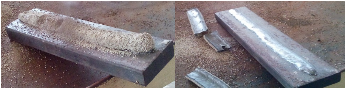
Fig. 3.2 Weld bead on plate surface (a) with slag layer deposit (b) after removal of slag layer [3]
