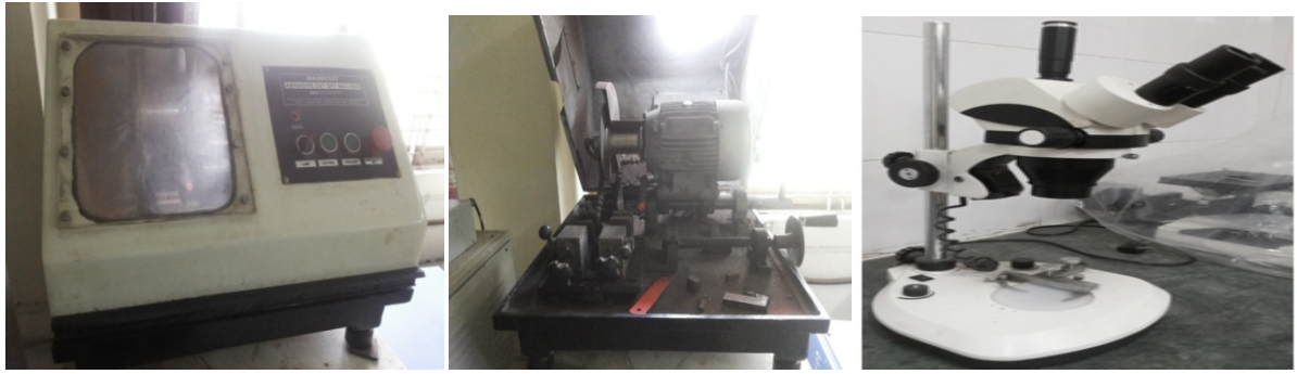
Fig. 3.4 (a) Abrasive cutting machine, (b) open cover shield, (c) stereo zoom microscope [3]
