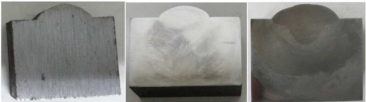
Fig. 3.2 Weld bead on plate surface (a) with slag layer deposit (b) after removal of slag layer [3]
