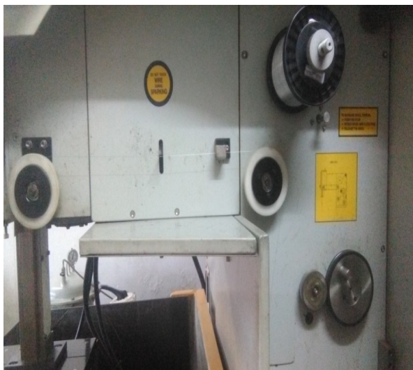
Fig. 3.9 (a) Wire feed mechanism with spool of wire and (b) operations in progress
