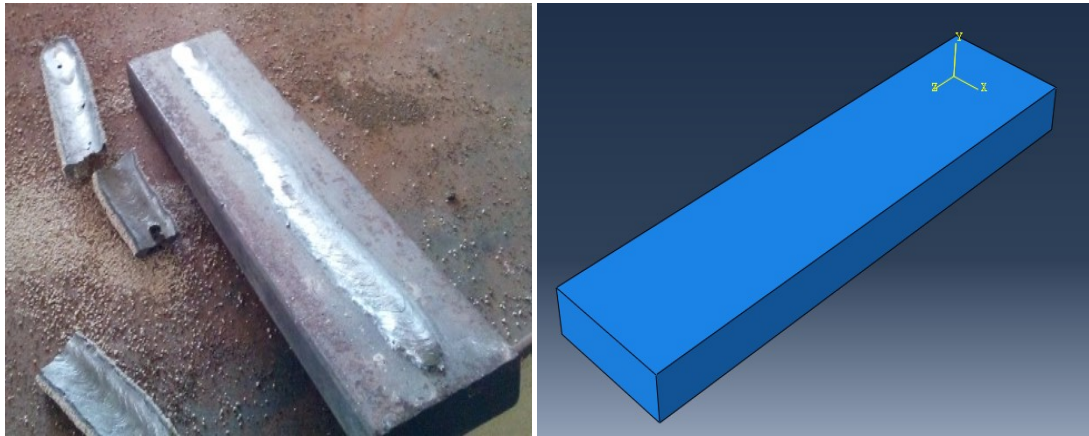
Fig 4.8 (a) Picture of weld bead on plate and (b) CAD model of plate
