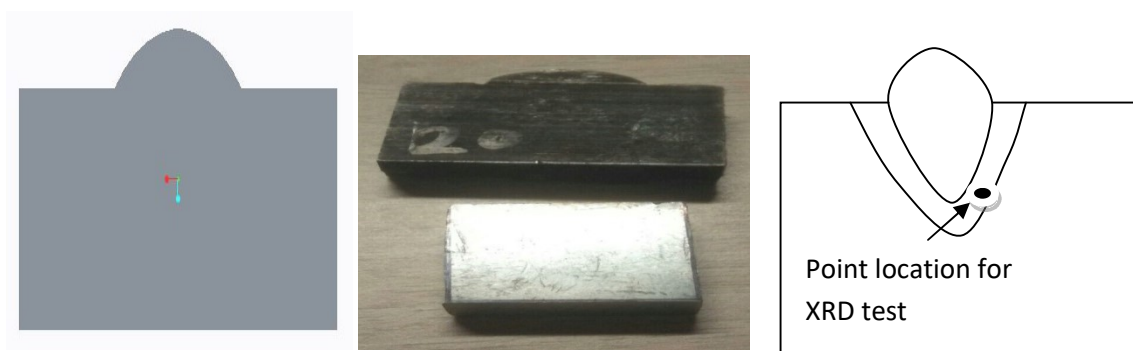
Fig. 3.10 (a) Schematic of work piece with weld bead, (b) Work piece before and after machining and (c) Schematic of HAZ and point location for XRD test
