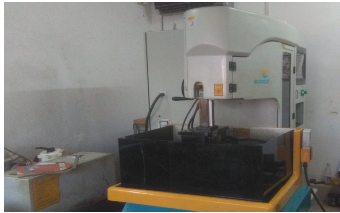
Fig. 3.7 ECOCUT WEDM with work piece on worktable and cover [Courtesy- Echo Tool Engineering, Bhopal]
