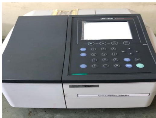
Figure 3.7: Spectrophotometer to get optimum density (OD 600 )
