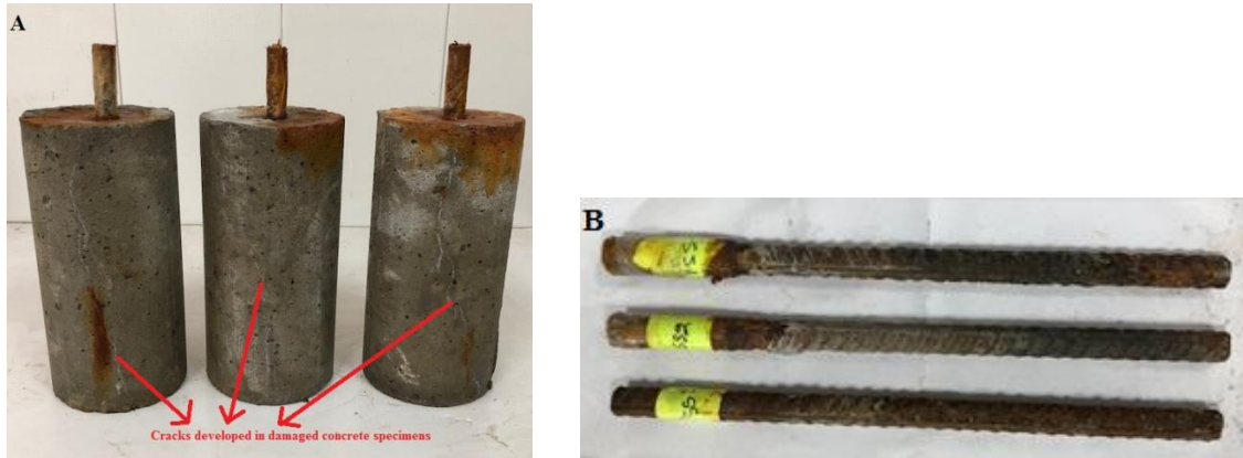
Figure 3.17: (A) Damaged specimens after corrosion, (B) Corroded bars
