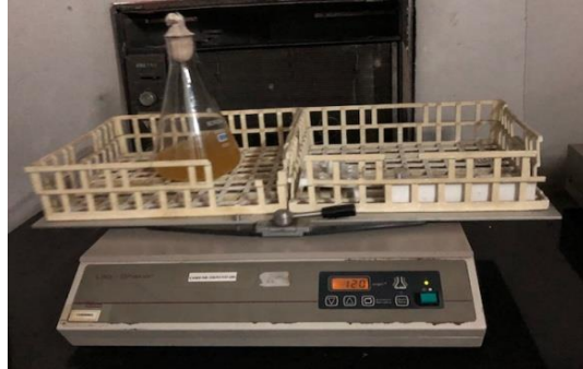
Figure 3.4: Shaker rotating at 120 rpm at 37°C
