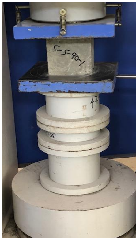
Figure 3.13: Compression testing machine of cube testing
