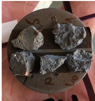
Figure 3.18: Coated sample for investigation under SEM
