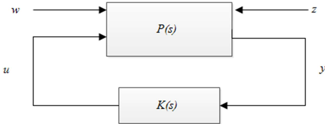
Fig.3.1. Closed-loop system via H_\infty control
