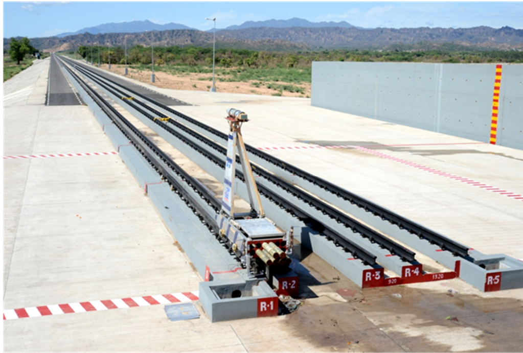
Figure1.2: The penta rail supersonic track which got augmented in the course of these studies
