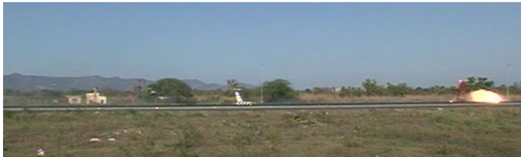
Figure 5.10: Plume due to retro-rockets, which affects the measurement of total pressure, was seen on the right end
