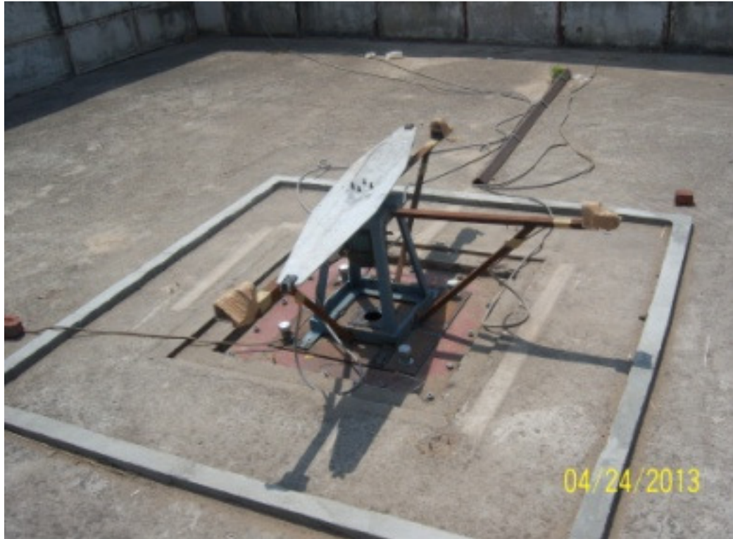
Figure 3.15: Test setup of rotating magnet.
