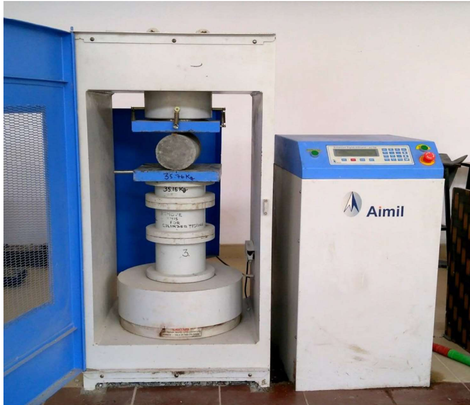
Fig. 3.12 Splitting tensile strength test set-up
