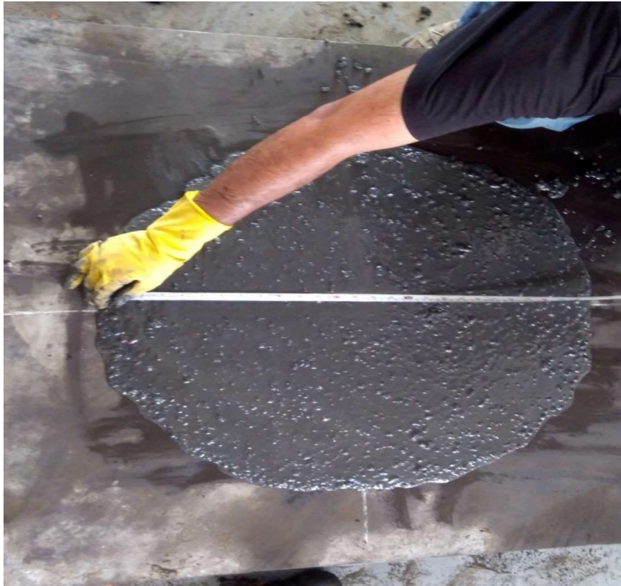
Fig. 3.7 Slump-flow test in progress
