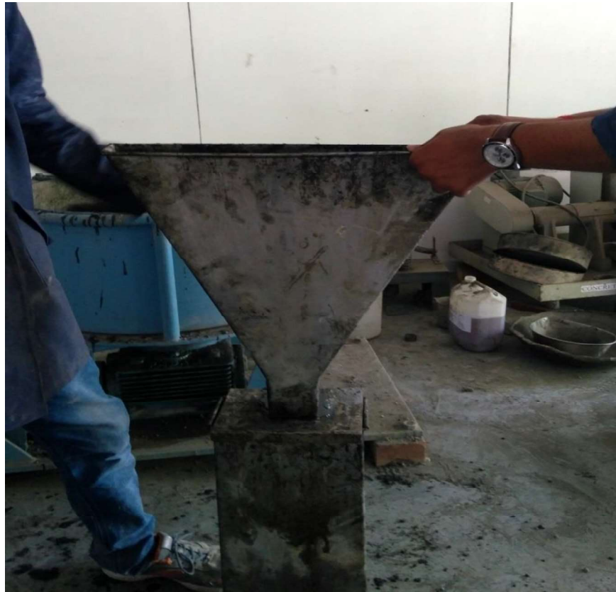
Fig. 3.8 V-funnel test in progress
