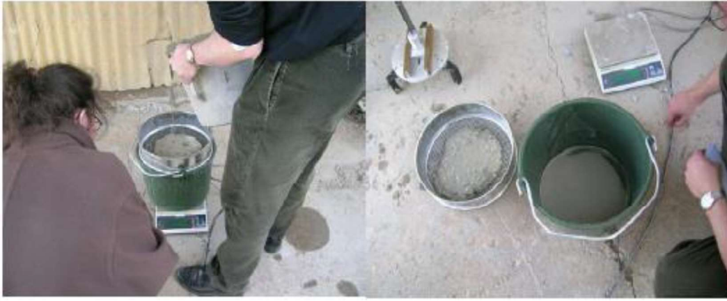
Fig.1.6 Sieve segregation test (EFNARC 2005 [10])
