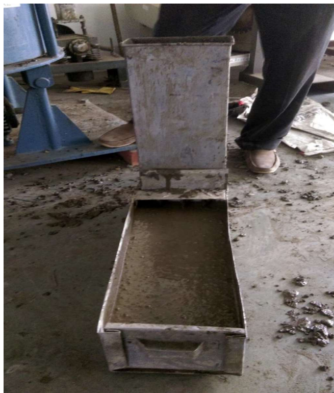
Fig. 3.9 L-box set-up (3 bar variant)
