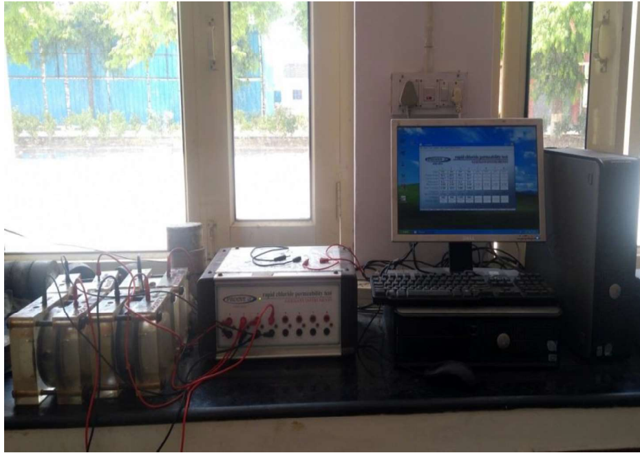
Fig. 3.13 Rapid chloride-ion permeability test set-up
