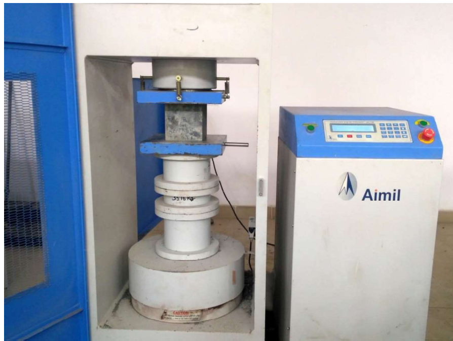
Fig. 3.11 Compressive strength test set-up
