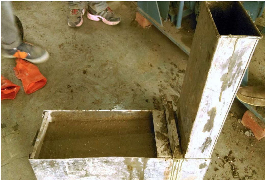
Fig. 3.10 L-box test in progress
