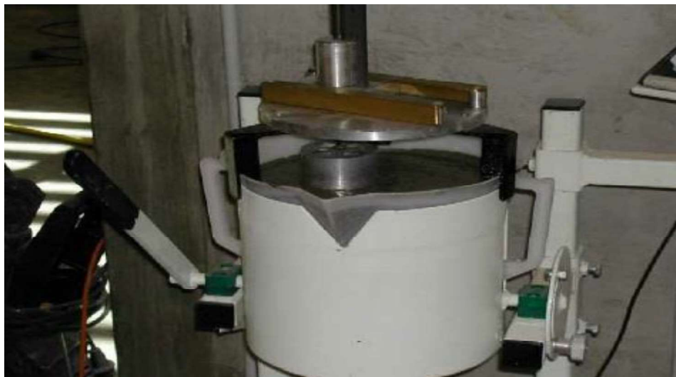
Fig.1.8 Penetration test apparatus (Source: www.researchgate.net )
