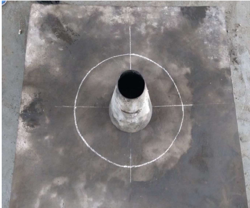
Fig. 3.6 Baseplate with slump-cone
