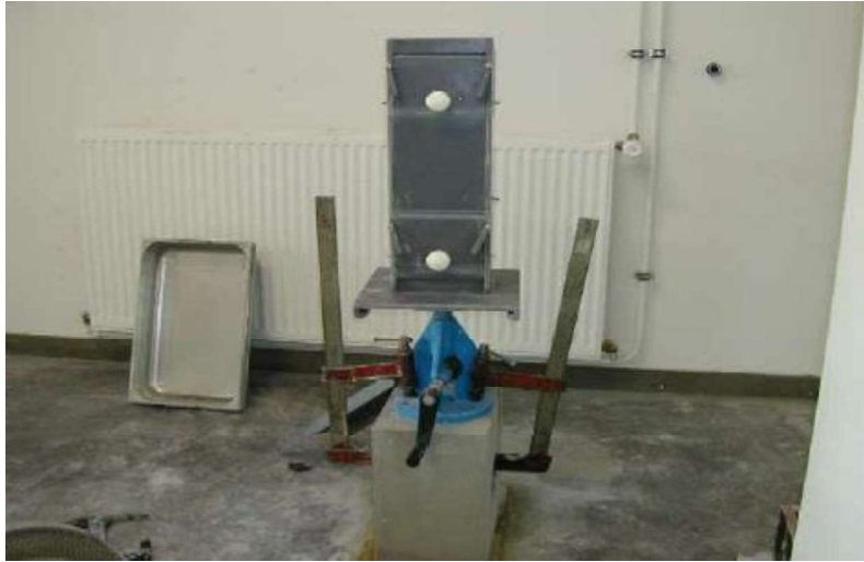
Fig.1.7 Settlement column segregation test (Source: www.researchgate.net )
