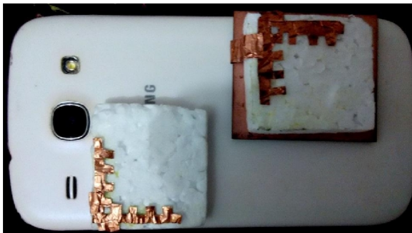
Fig. 4.11 Fabrication of the proposed MIMO antenna system in comparison to Samsung 4.5 inch mobile phone.
