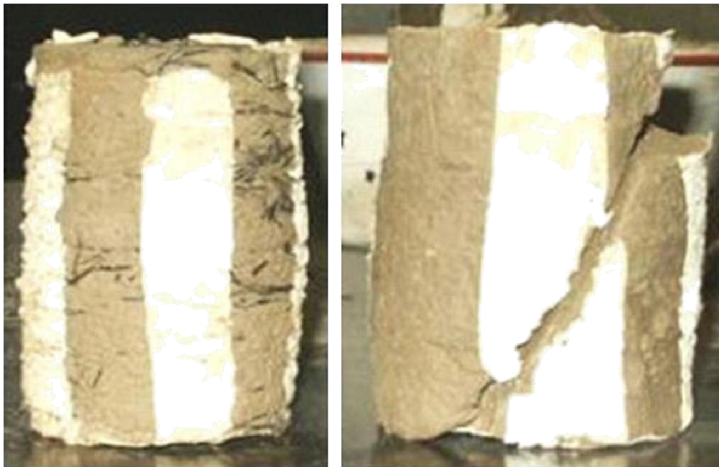
Fig.2.26 Effects of PP fiber inclusions on the soil
