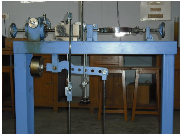
Plate 3.3 Photograph showing direct shear test set up
