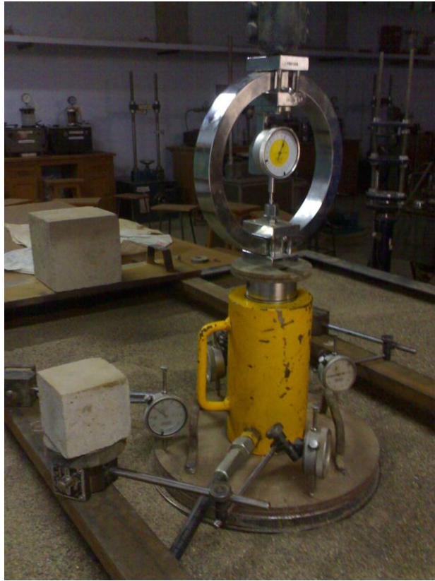
Plate 3.8 Photograph of dial gauges for measurement of settlement of a plate
