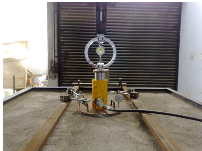
Plate 3.6 Photograph of large scale plate load test (1.5m X 1.5m X 1.0m)
