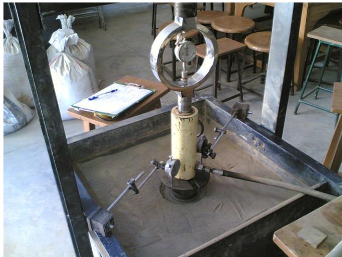
Plate 3.5 Photograph of small scale plate load test (0.6m X 0.6m X 0.6m)
