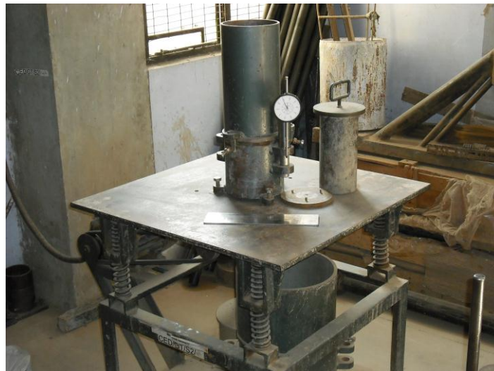
Plate 3.4 Photograph showing relative density test set up
