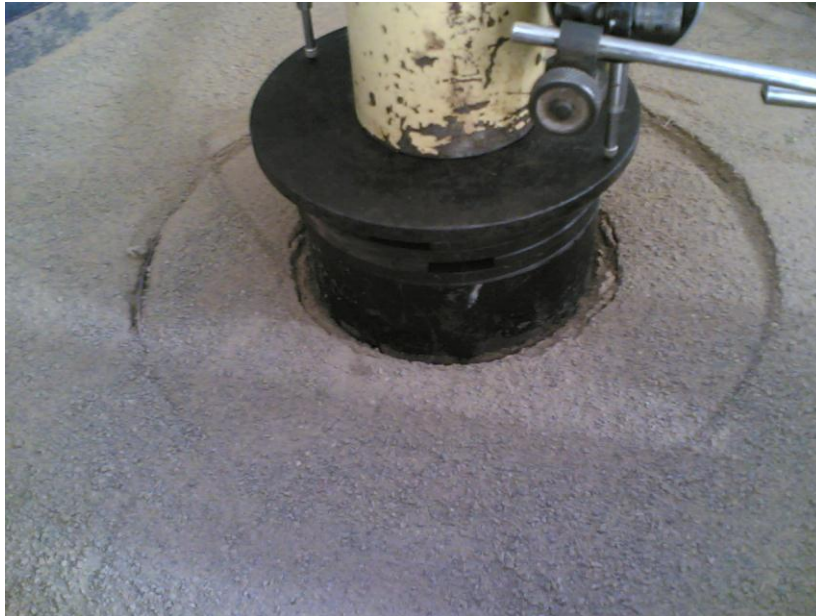
Plate 4.4 Photograph indicating the settlement of the plate while the cell is unaffected for D=150\text{mm}
