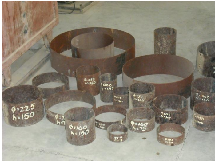
Plate 3.2 Photograph showing confining cell of different diameters and heights
