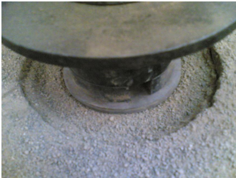
Plate 4.3 Photograph indicating cell, soil, and footing settled together for D=150\text{mm} ( d/D=1.5 )
