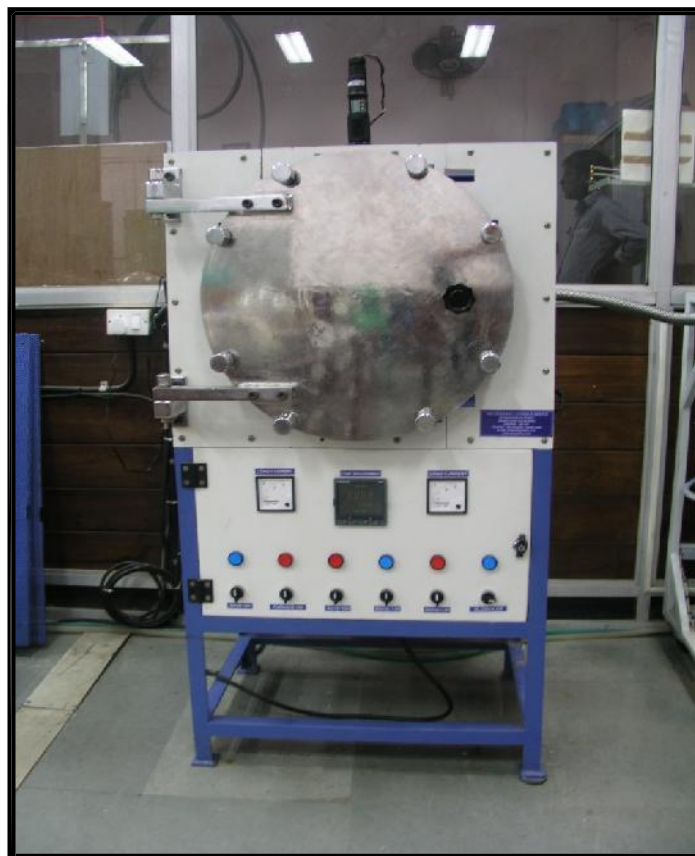
Fig 3.10: Microwave furnace used for sintering Cu-Cr alloy
