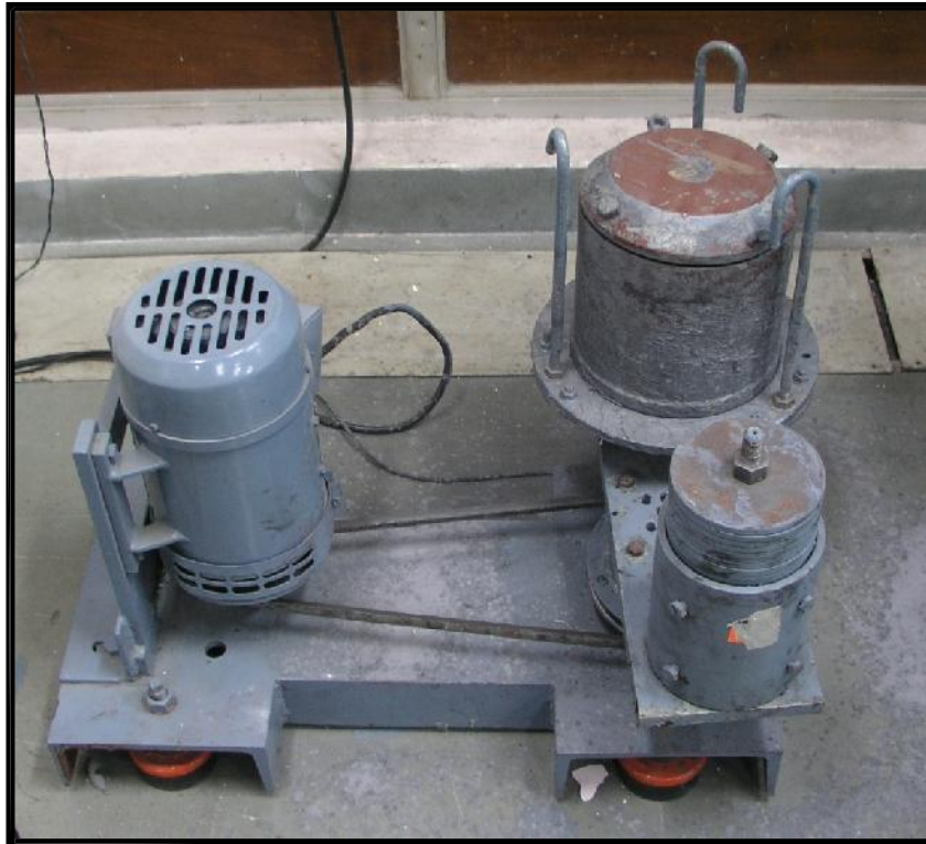
Fig. 3.1: Planetary Ball Mill used for Mechanical Milling
