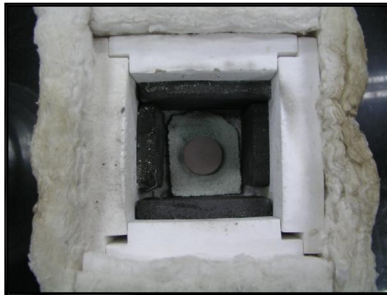
Fig 3.11: Loading of green compact in a insulation package used for microwave furnace
