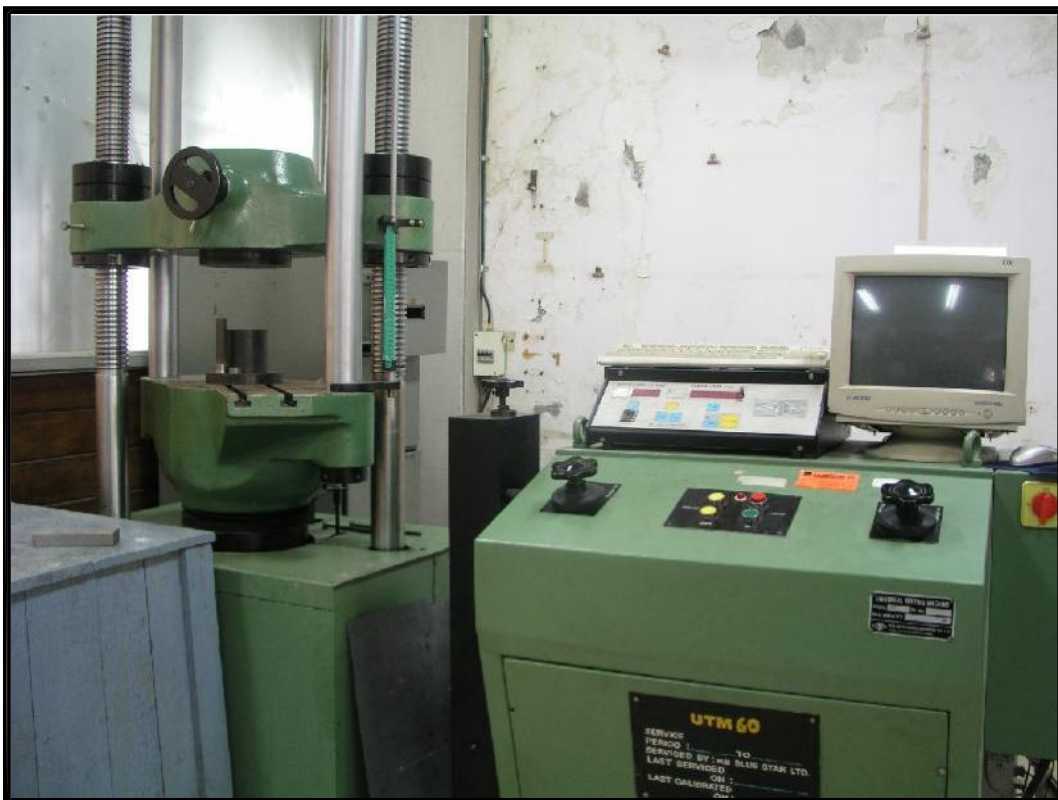
Fig. 3.3: UTM 60 uniaxial semi-automatic hydraulic press
