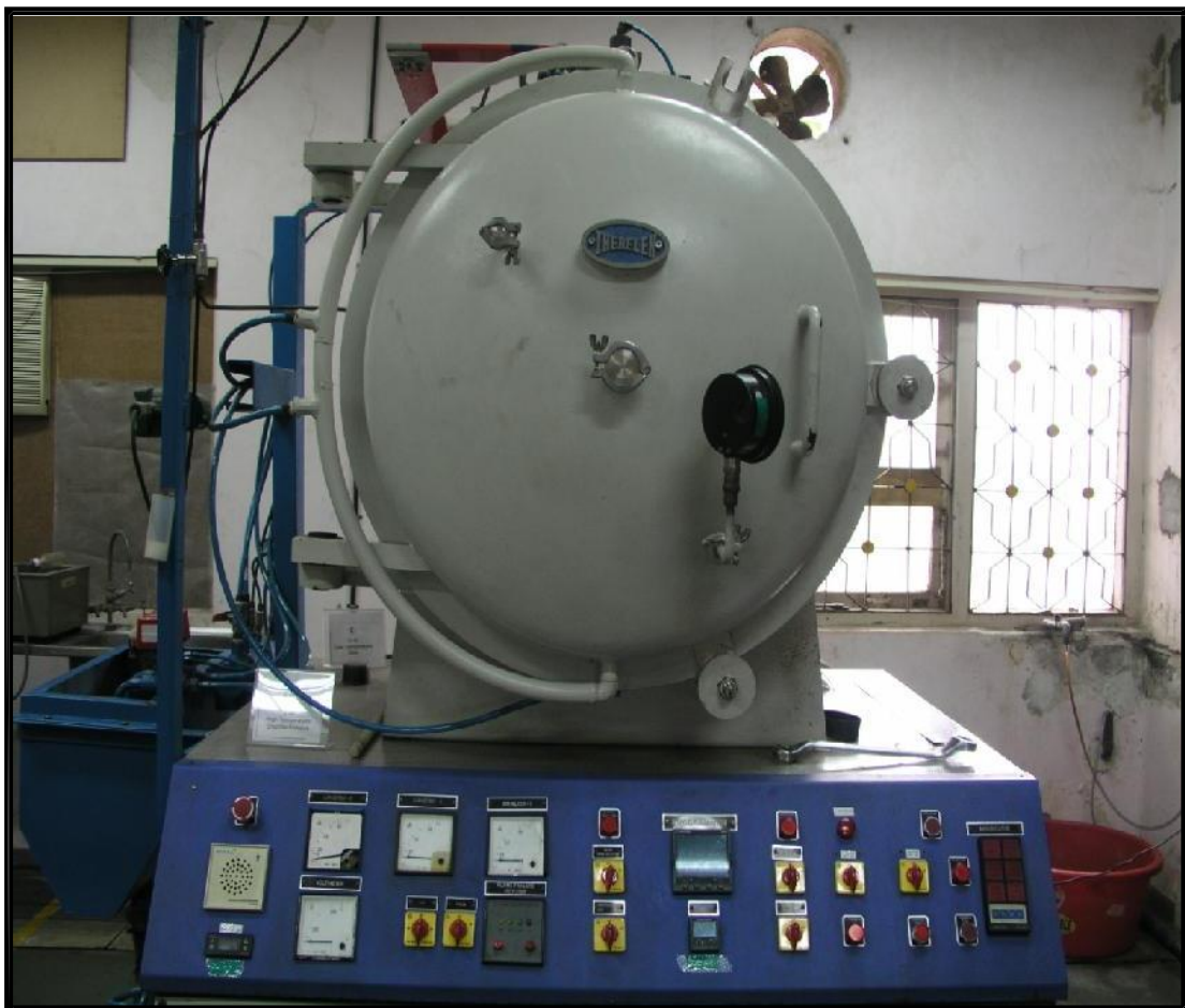
Fig. 3.12: Conventional high temperature graphite furnace
