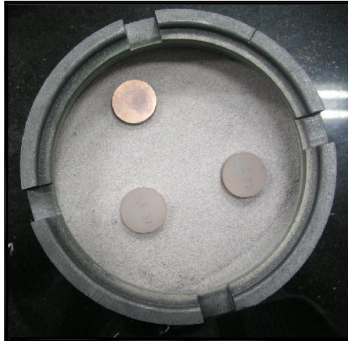
Fig. 3.13: Loading of green compacts in graphite crucible used for conventional furnace.
