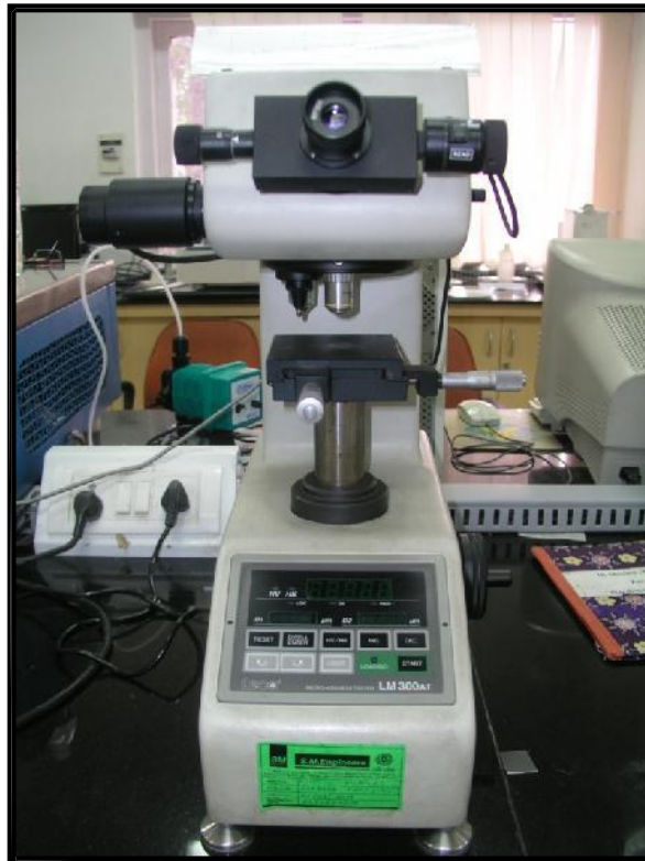
Fig. 3.14: Leco LM 300 AT hardness tester
