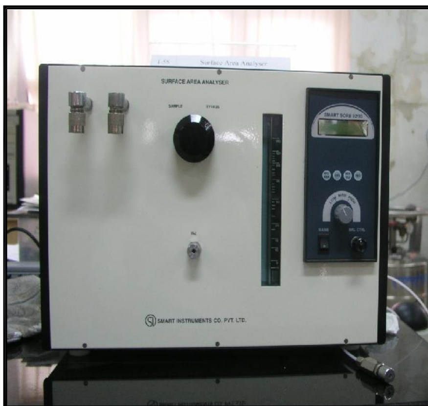
Fig. 3.2: Smart Sorb 92/93 surface area analyzer
