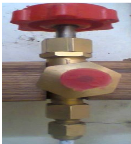
Fig 4.4: Hand Operated Expansion Valve
