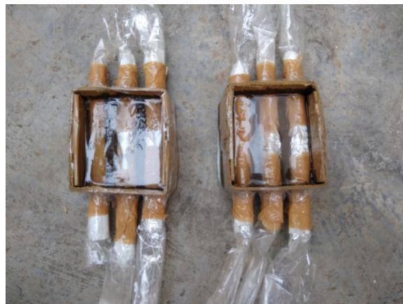
Figure 5.5 Cardboard moulds used to make specimens
