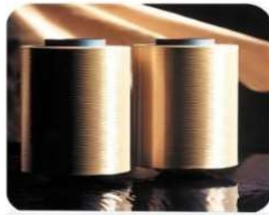
Figure 1.11 Aramid fibres roll [2]
