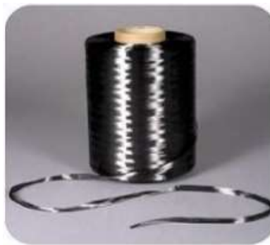
Figure 1.12 Carbon fibres roll [2]
