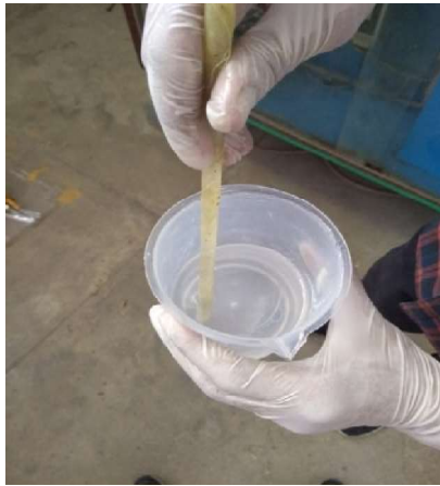
Figure 5.4 Mixing of epoxy resin and hardener
