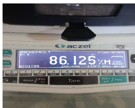
Fig2 - measuring the moisture content
