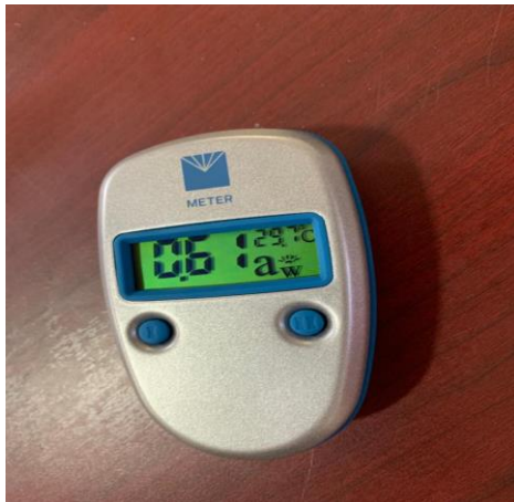
Fig11- Measuring the water activity of ber slices
