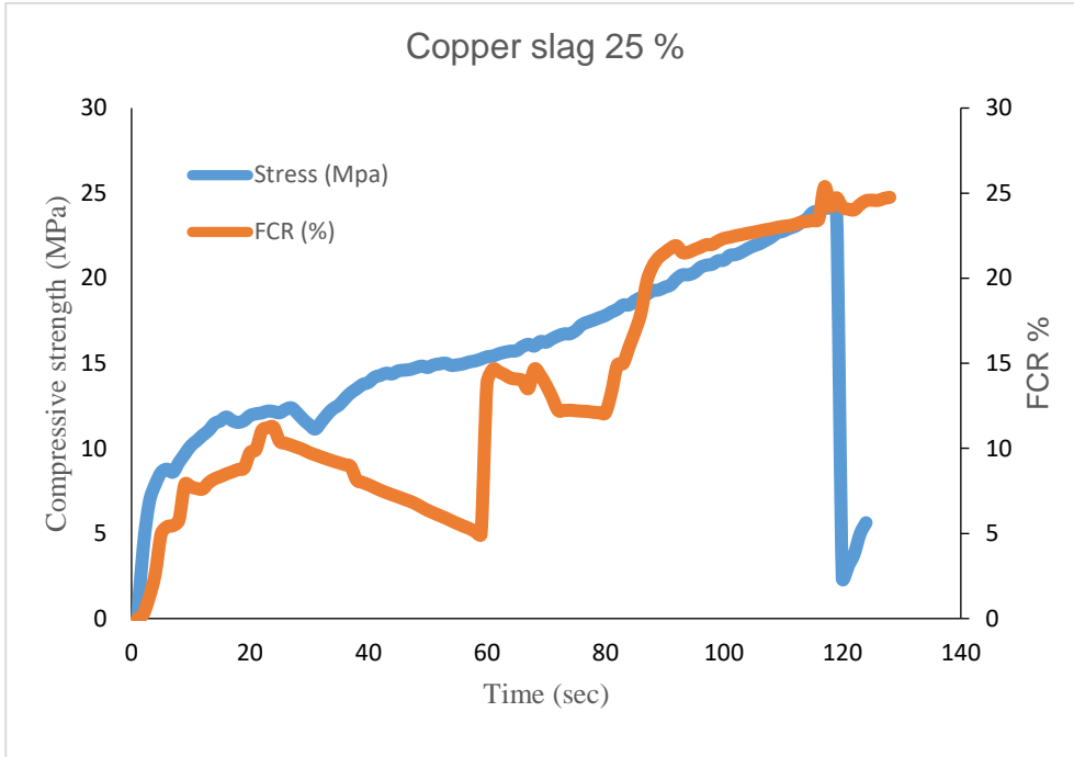
Figure 4.9. Compressive strength vs FCR tested for 56 days
