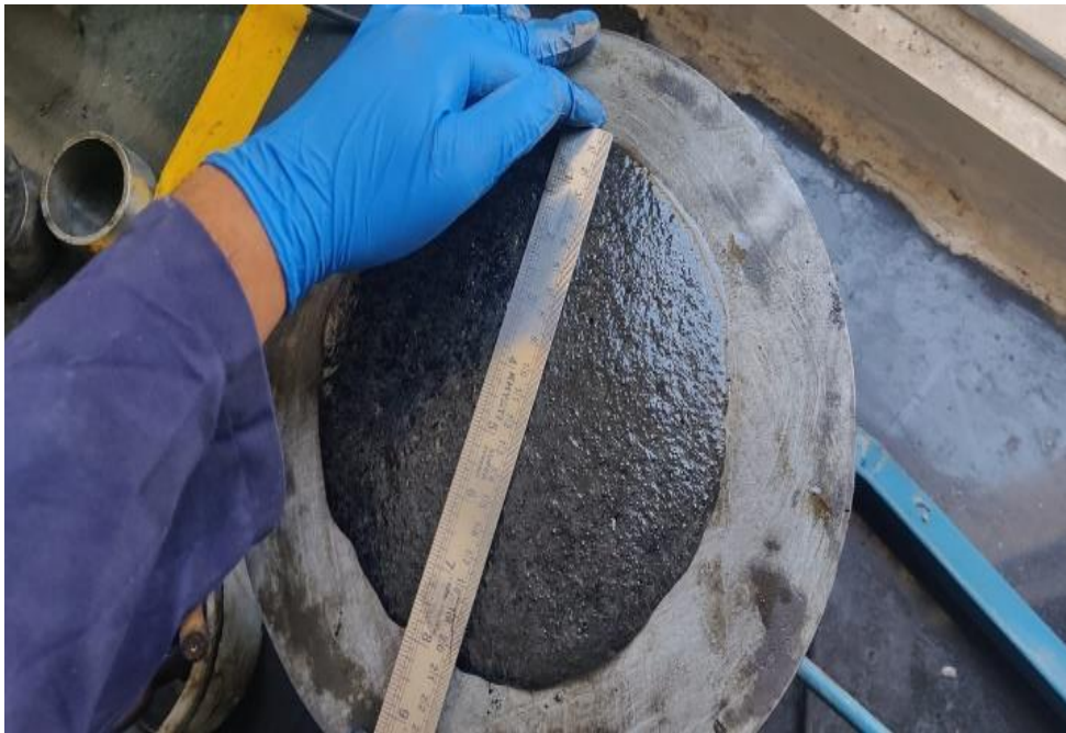
Figure 3.9. Measurement of workability
