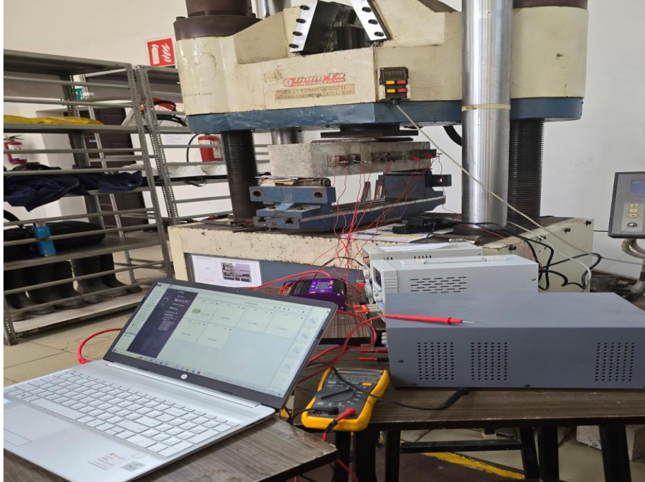
Figure 3.14. Setup for Beam testing
