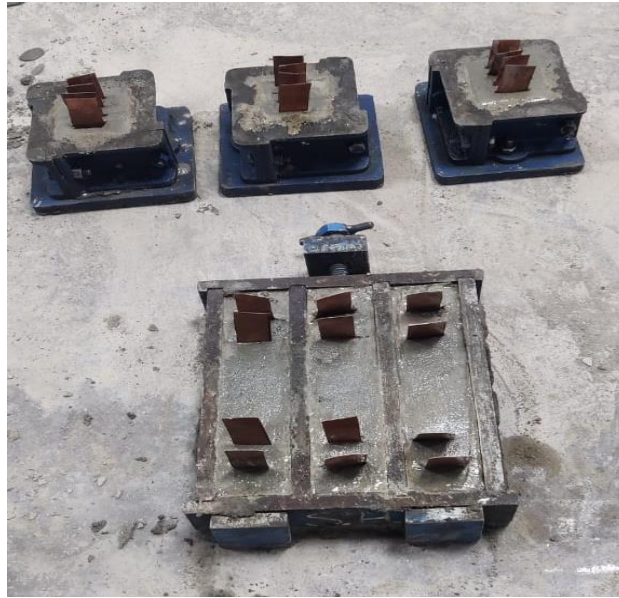
Figure 3.2. Copper plate's embedment in cube and prism samples
