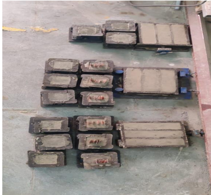
Figure 3.4. Casting of Cubes & Prism
