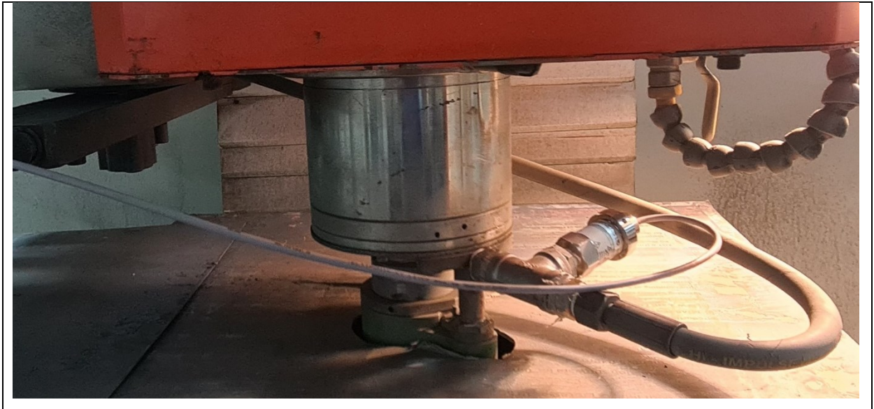
Figure 3.5: BT40 coolant inducer mounted on the spindle of 3-axis vertical CNC milling centre with the pressure sensor (PS2) mounted at the inlet of BT40 coolant inducer.
