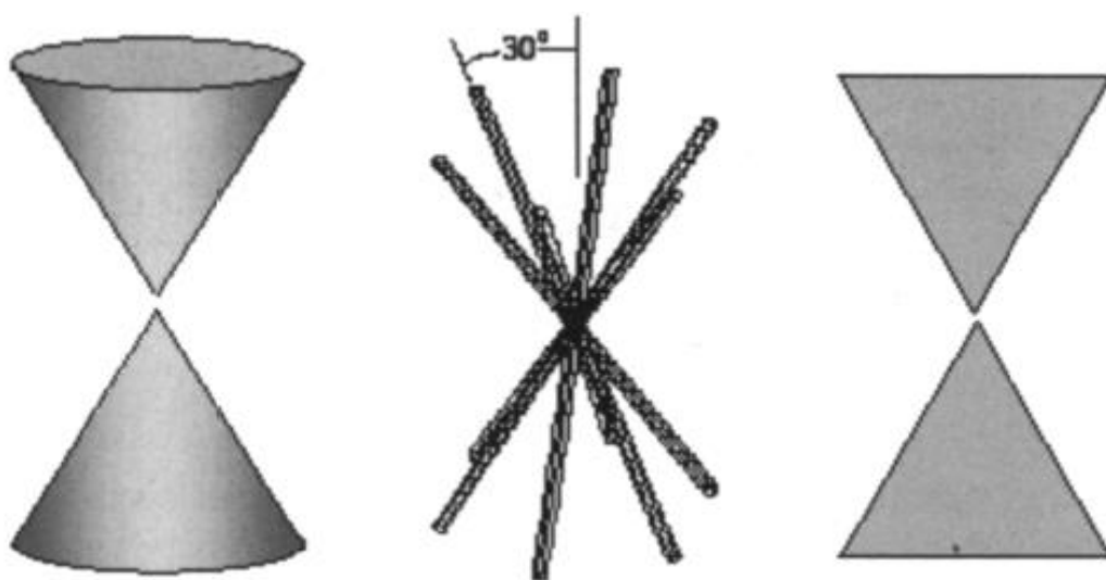
Fig 1.8: Bowtie and biconical antennas[10].
