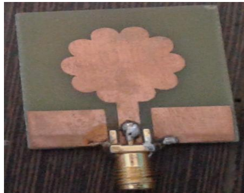
Fig 7.3 Fabricated Fractal Flower Antenna
