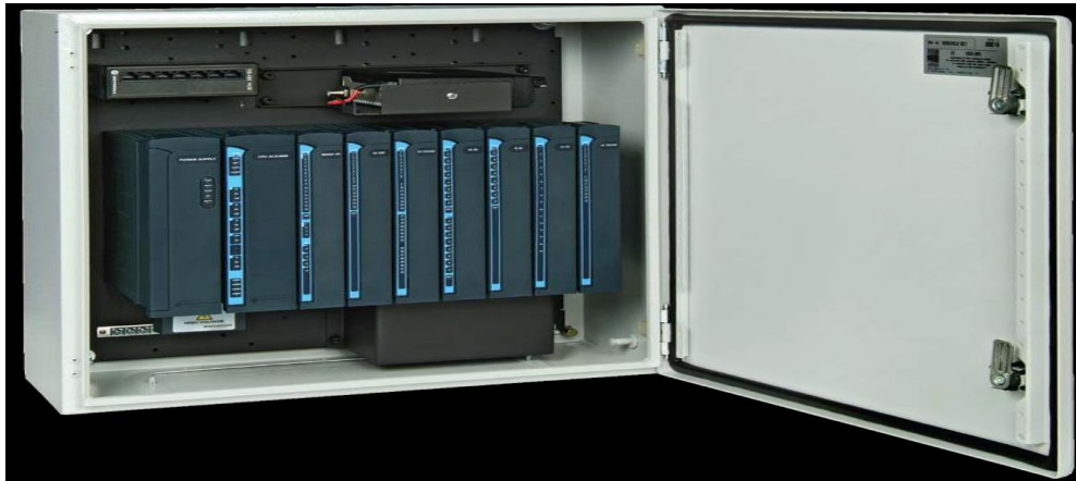
Figure 1.2 Motorola's ACE3600 RTU [16]
