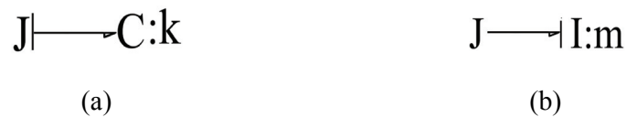
Fig. 3.4 Representation of (a) capacitive and (b) inductive element along with their causality
