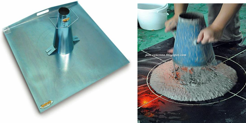
Fig 2.2: Slump cone test (Ferraris, 1999)
