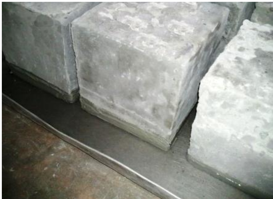
Fig. 4.14: Specimen immersed in water at a height of 5 mm.
