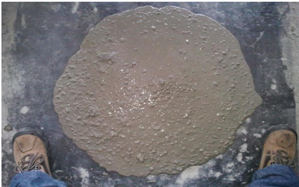
Fig. 4.1: Slump flow test.
