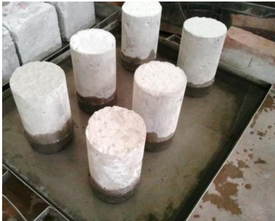
Fig.4.16: Specimen dipped in Sodium Sulfate solution.
