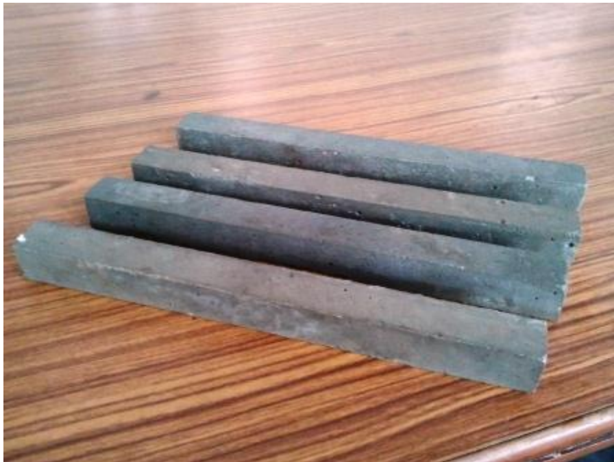
Fig. 4.9: Specimens for Shrinkage.
