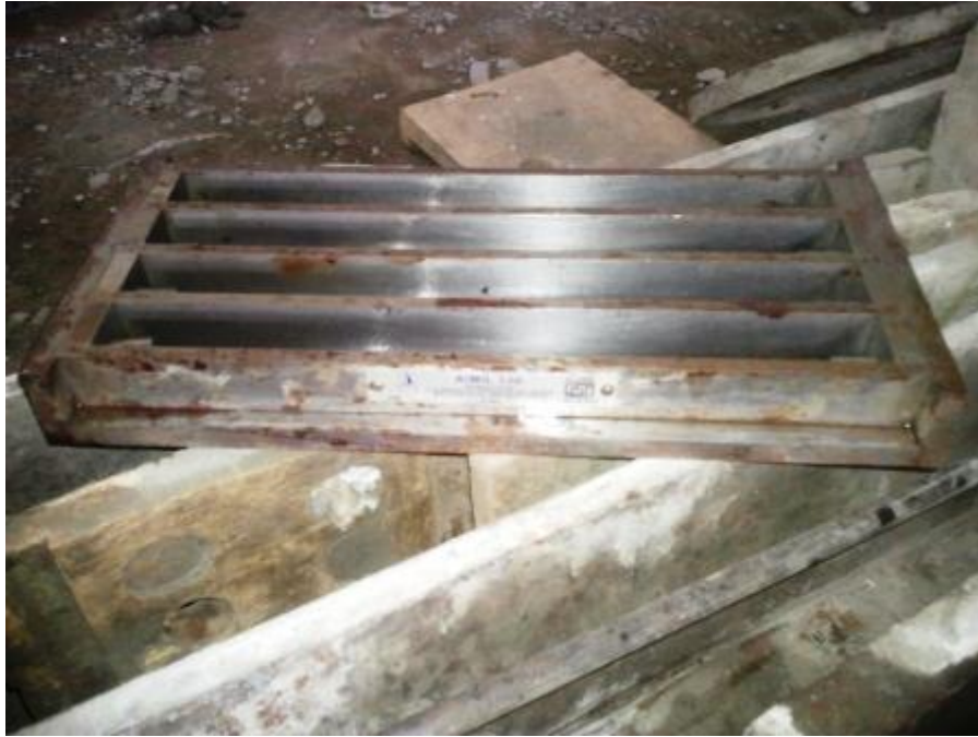
Fig.4.6: Shrinkage bar mould.
