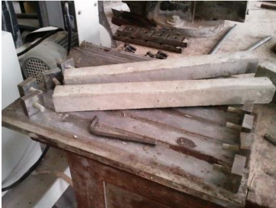
Fig. 4.8: Specimens for Shrinkage.
