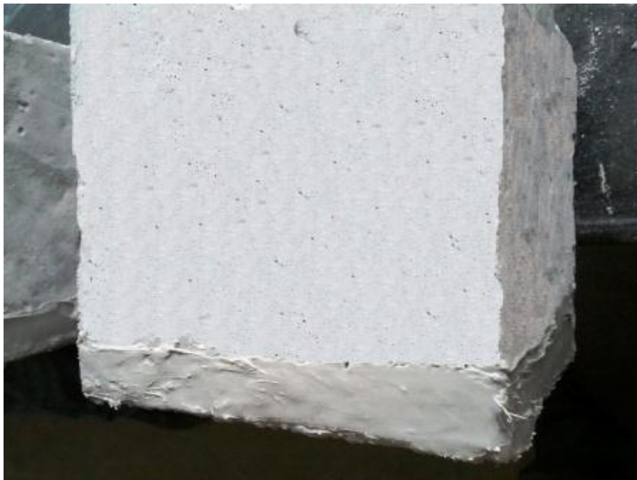
Fig.4.12: Specimen Sealed with water seal.
