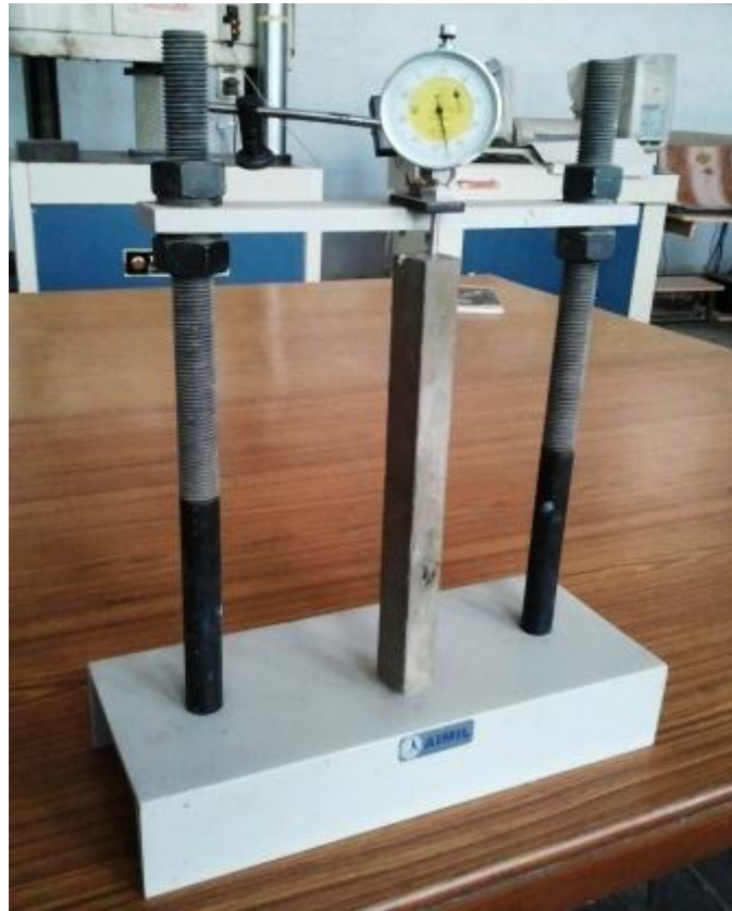
Fig. 4.10: Length measurement with Shrinkage tester.
