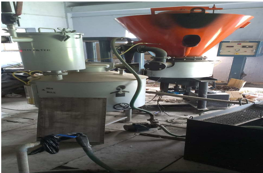
Figure 5.16: Complete gasifier unit
