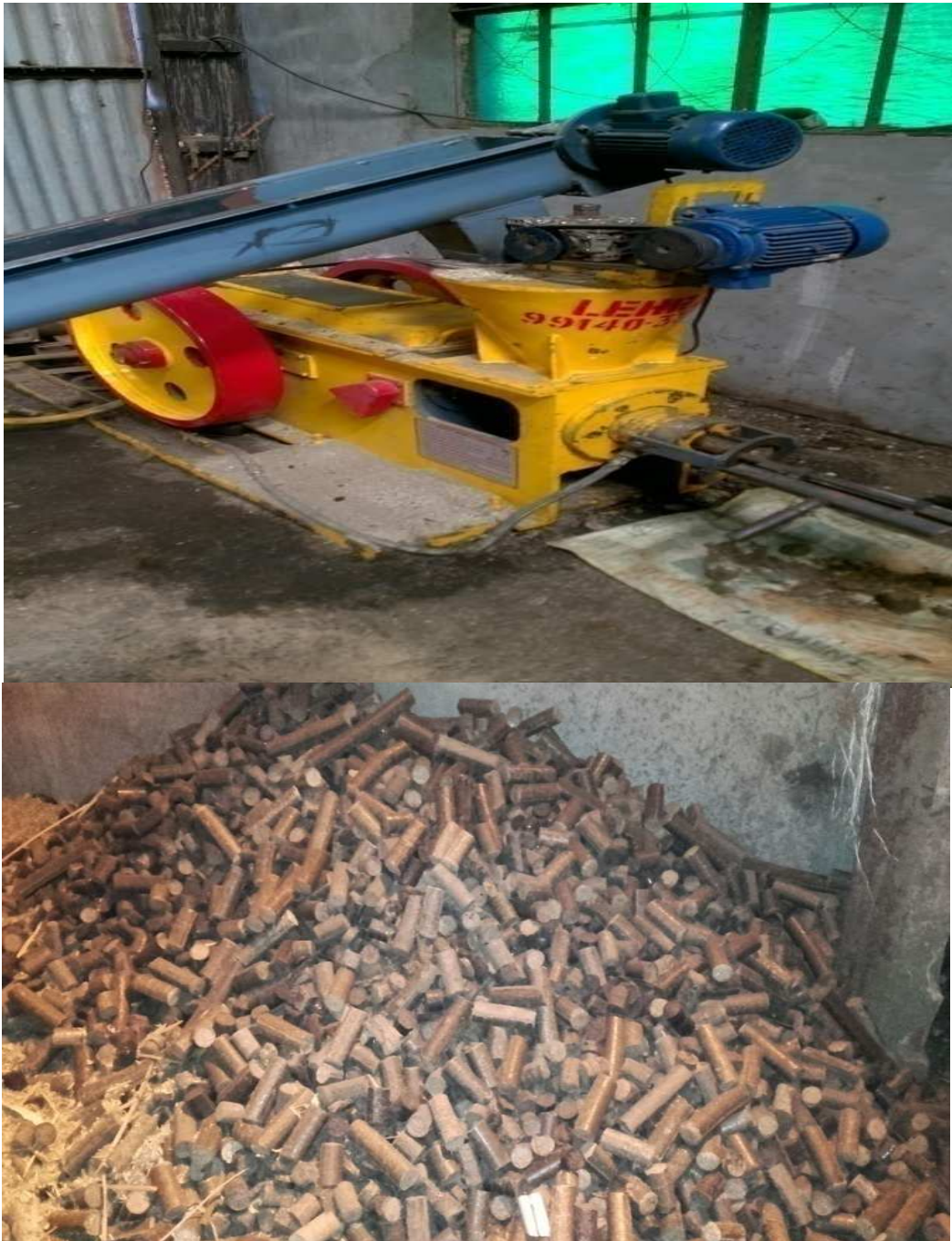
Figure 5.13: Briquette press and production of briquettes
