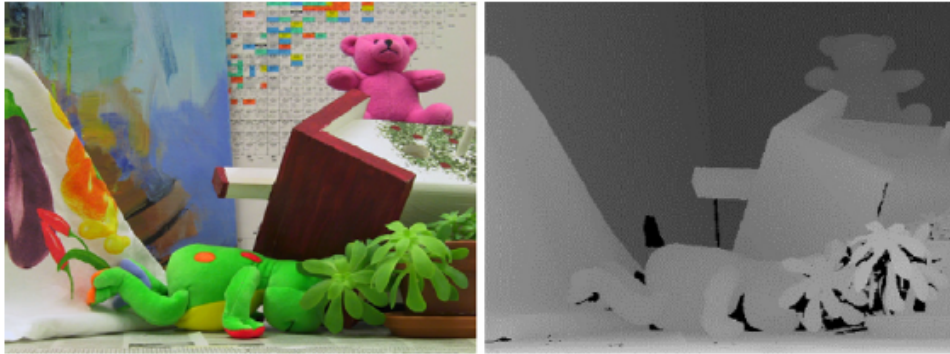
Figure 1.1: Tsukuba 2D camera image and depth map belonging to the image. Pixels go darker as the depth grows.
