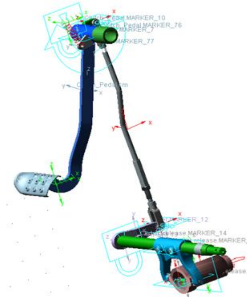
Fig. 4.1 ADAMS analysis model of clutch release fork
