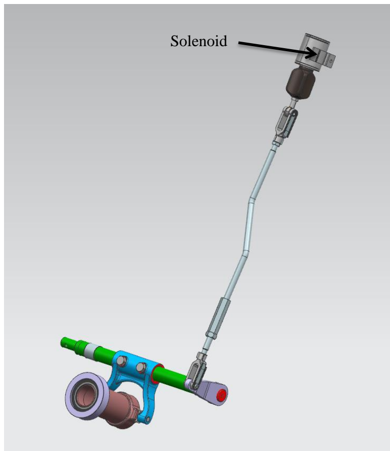
Fig. 5.3 New innovative model of clutch release fork with electric solenoid
