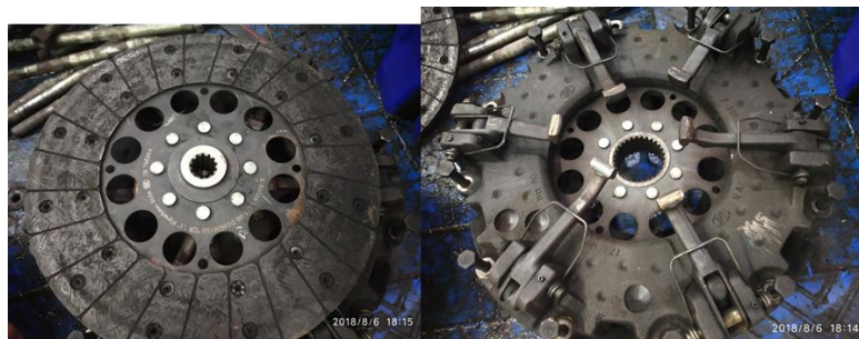
Fig. 1.2 Dual clutch model [1]
