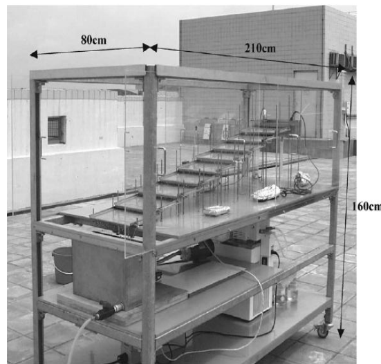
Fig-2.4 Cascade reactor
