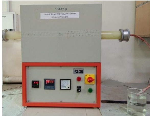
Figure 2.4: Tabular furnace used for sulfurization
