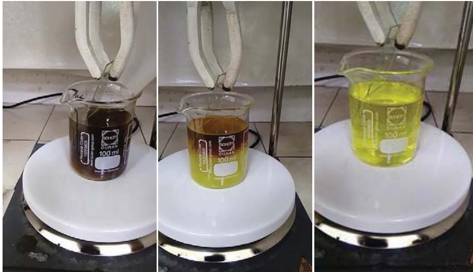
Figure 2.3: The color of bath solution changes with time after adding thiourea in the mixture of both stock solutions.
