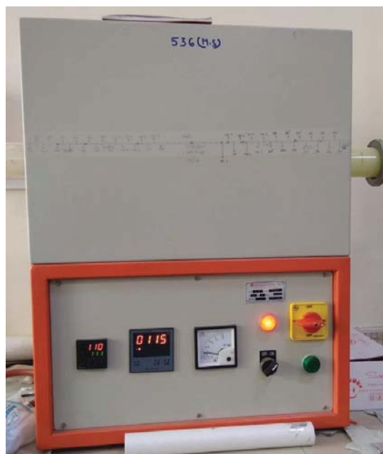
Figure 2.5: Photograph of tubular furnace used for sulfurization process.
