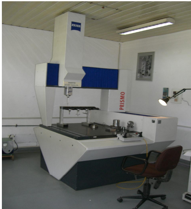
Figure 3.2: CMM used for Measurement of Worn Die
