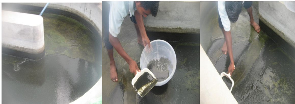
Algal slurry was mixed with the carrier material (fly ash)
