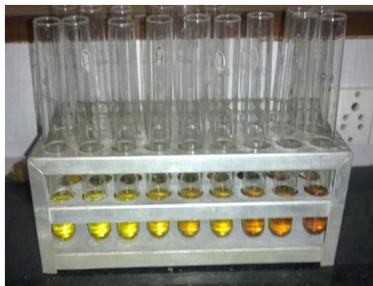
Figure 4: Test tubes showing increasing intensity of colour formed during sucrose estimation by DNSA method
