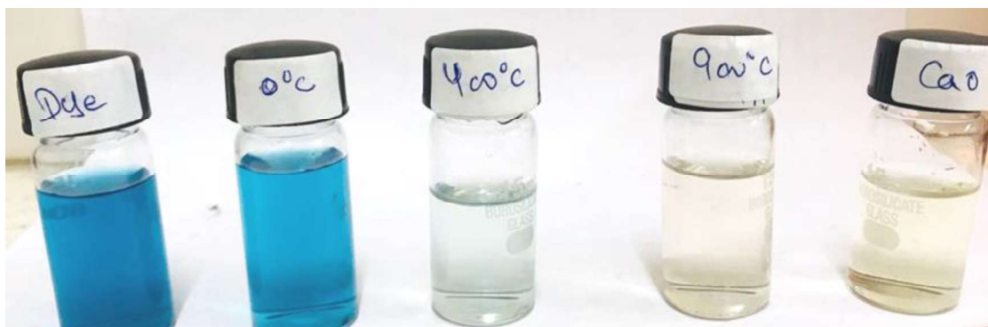
Fig.17: Comparative study of (RMP-TWB) with commercial available CaO at various temperature and observed color transformation from blue to transparent.
