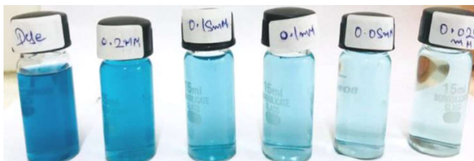
Fig.15: Effect of MG dye concentration and observe colors transformation from blue to transparent.
