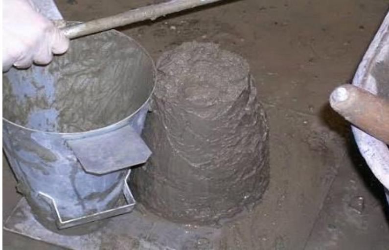
Fig. 3.2 : Slump Test of Concrete
