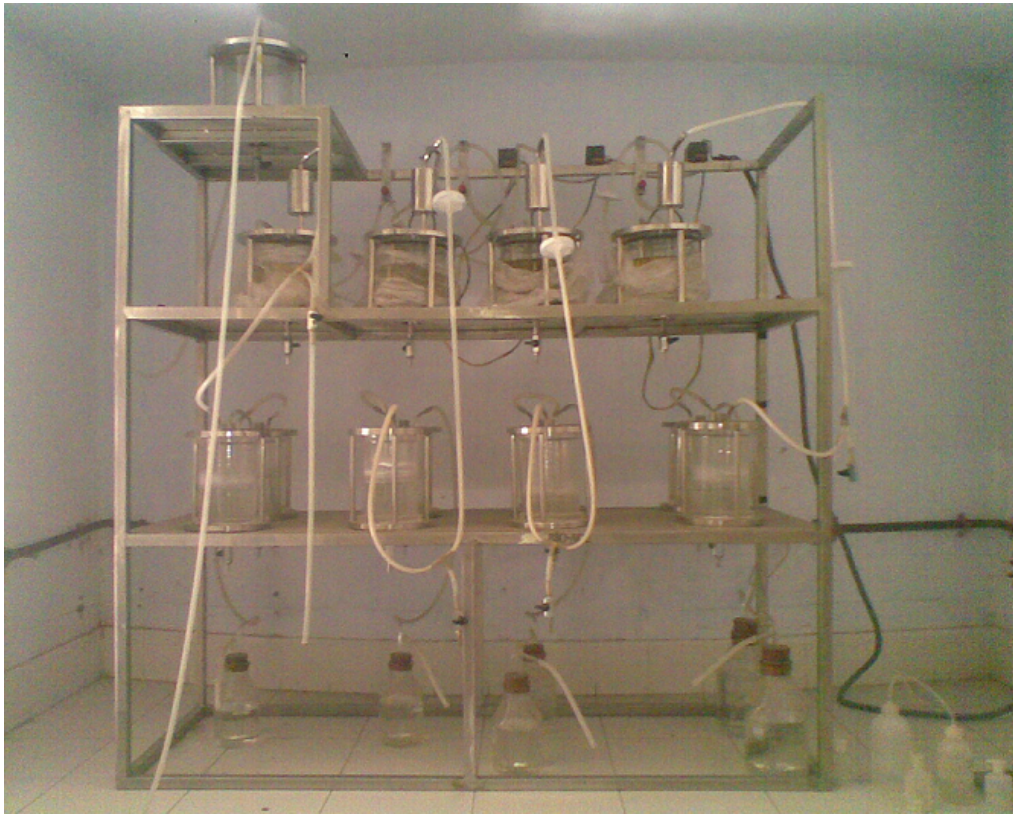
Fig 4.14 Biodegradability test apparatus according to standard ASTM D5338 (2003)
