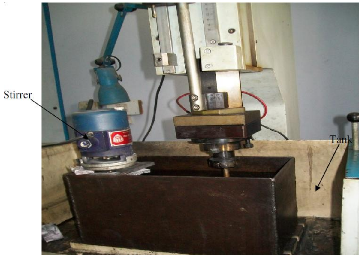
Figure 3.3 Dielectric Tank along with stirrer [Courtesy by: NTM Lab, Thapar University, Patiala]
