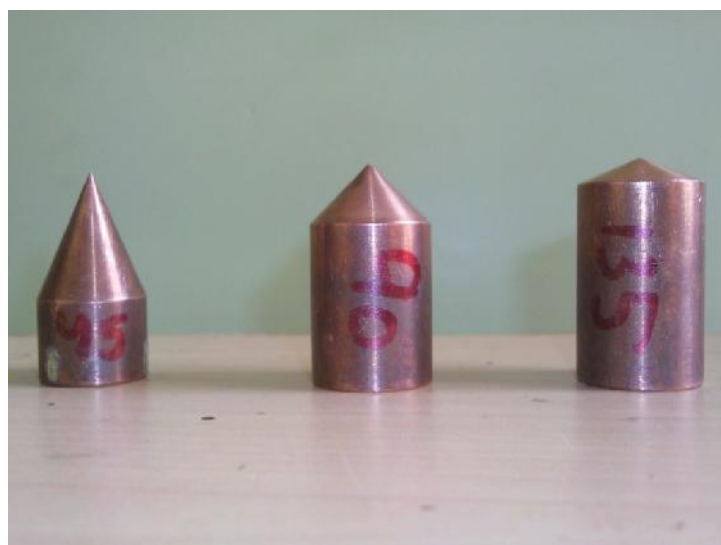
Figure 3.5 Workpiece after machining (a) AISI 304 (b) ALLOY (c) MMC
