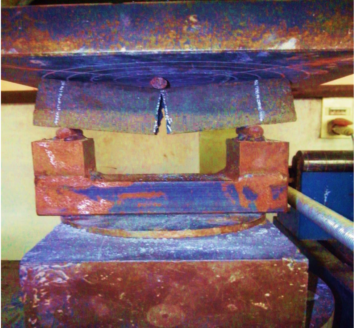
Fig. 3.6 Failure of Sample during Flexural Testing under Three Point Loading
