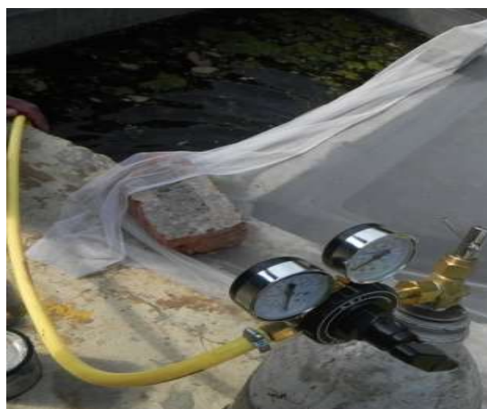
Fig 3.4: Supply of CO 2 in the algae- pond
