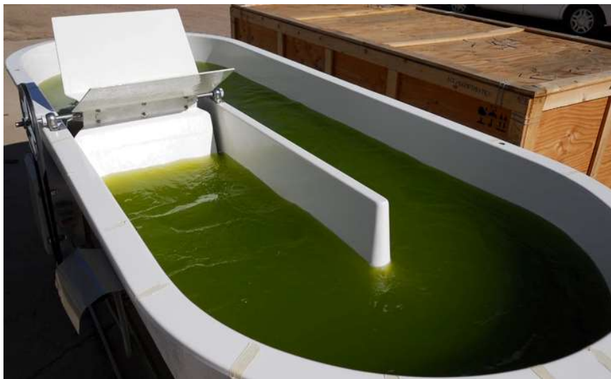
Fig 2.2: Raceway pond (source- Google images)
