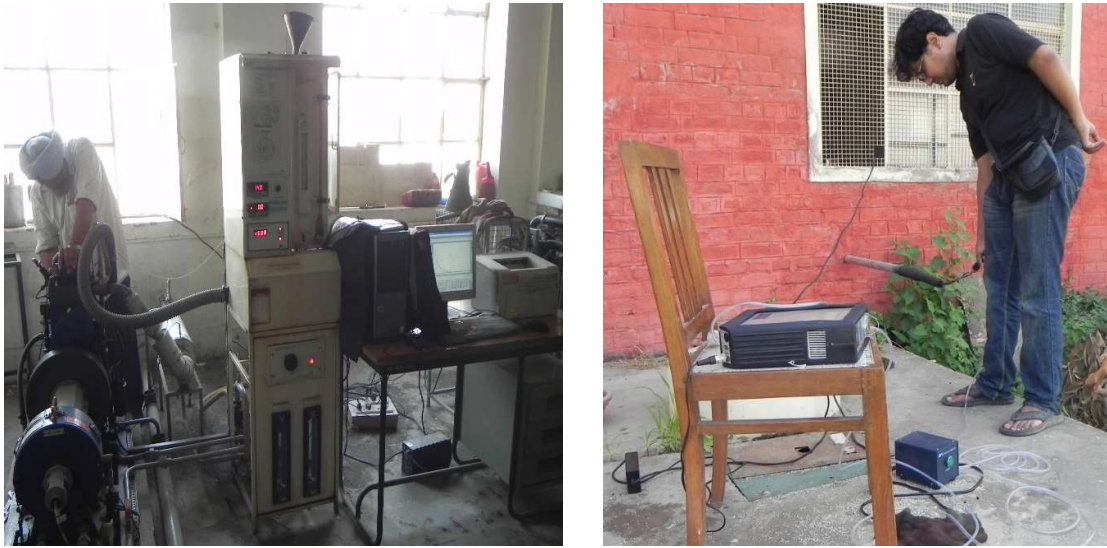
Fig 3.24: Operation of engine and AVL 444 digas analyser to examine the emission of algal biodiesel- petro- diesel blends
