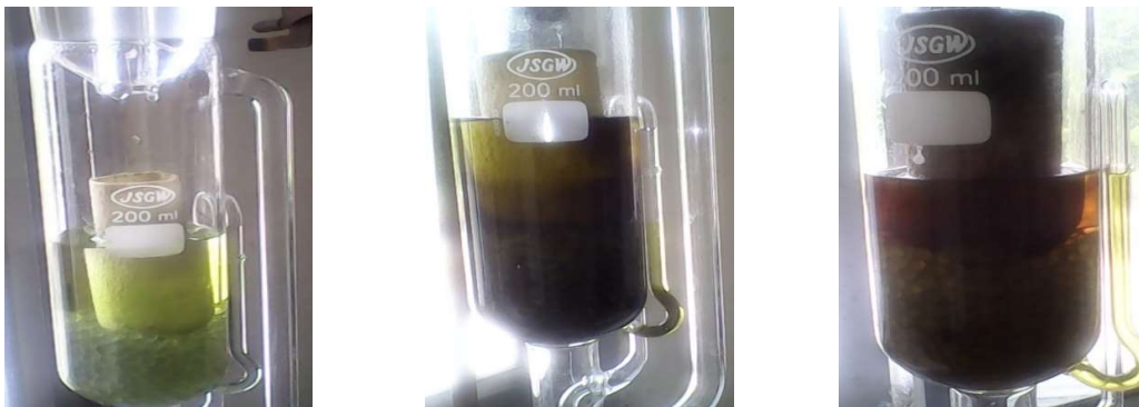
(a) (b) (c) Fig 4.24: Oil extraction with (a) methanol; (b) hexane; (c) acetone
