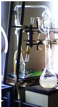
Fig 3.5: Determination of nitrogen of pond water using Kjeldahl apparatus
