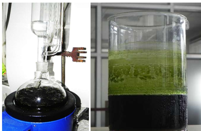
Fig 4.25: Oil extraction by submerging the algae directly in solvents
