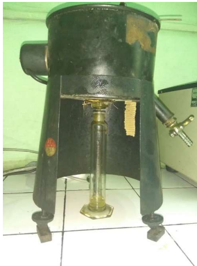
Fig 3.15: Redwood viscometer used for measuring the viscosity of the algal biodiesel
