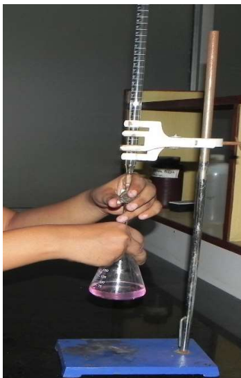
Fig 3.19: Titration for the estimation of acid number of algal biodiesel
