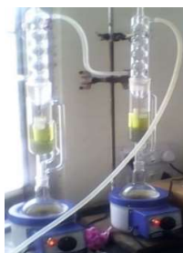
Fig 3.12: Solvent extraction of algal oil with Soxhlet apparatus
