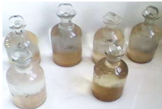
Fig 3.8: Estimation of DO of pond water
