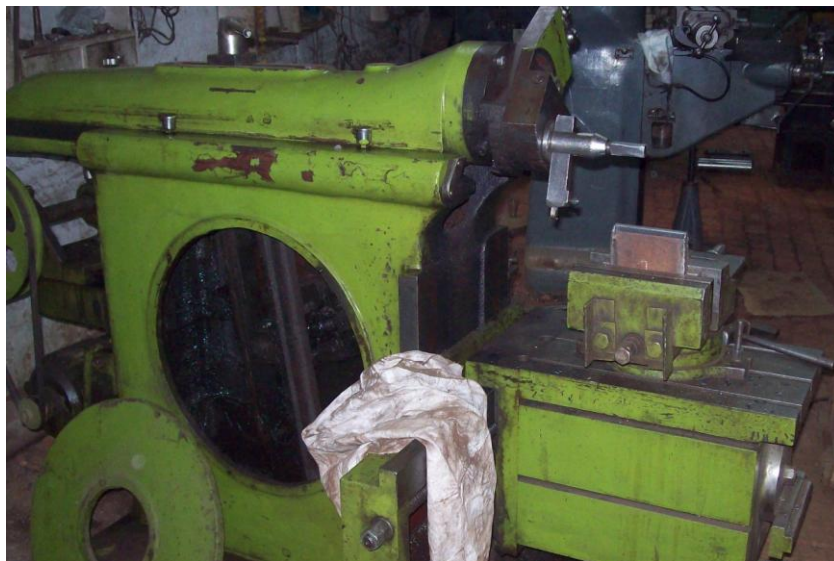
FIGURE 3.7- Making chamfer on corner of plate
