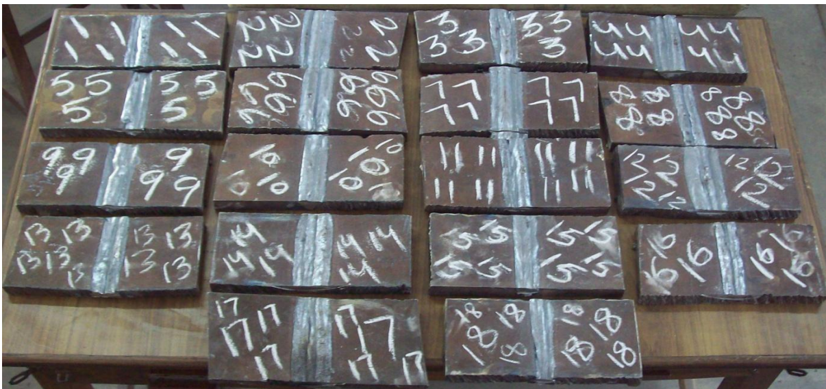
FIGURE 3.14- Welding on plates
