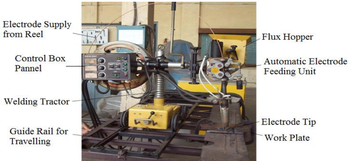
FIGURE 1.4- Set up of SAW process
