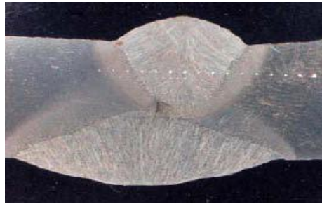
FIGURE 1.12- Insufficient penetration and excessive reinforcement, also misaligned [4]
