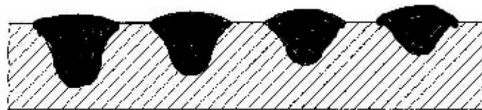
FIGURE 1.6- Effect of variation in welding speed on weld bead profile [4]
