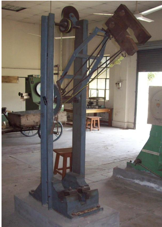
FIGURE 3.28- Charpy toughness test machine (Courtesy: Strength of Material Lab, Thapar University, Patiala)
