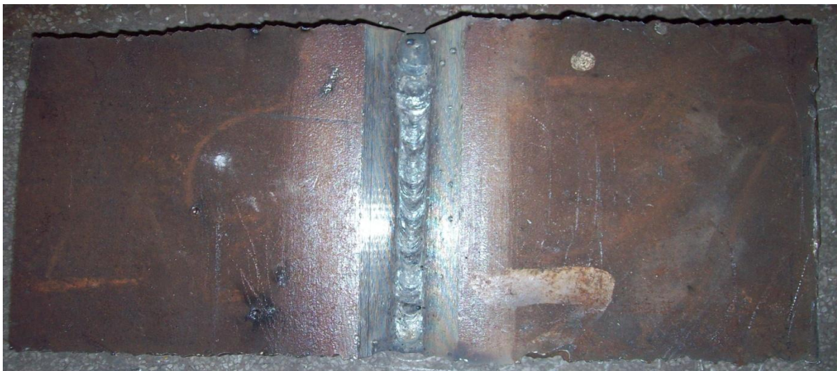
FIGURE 3.11 -Root layer between grooves of plates through SMAW
