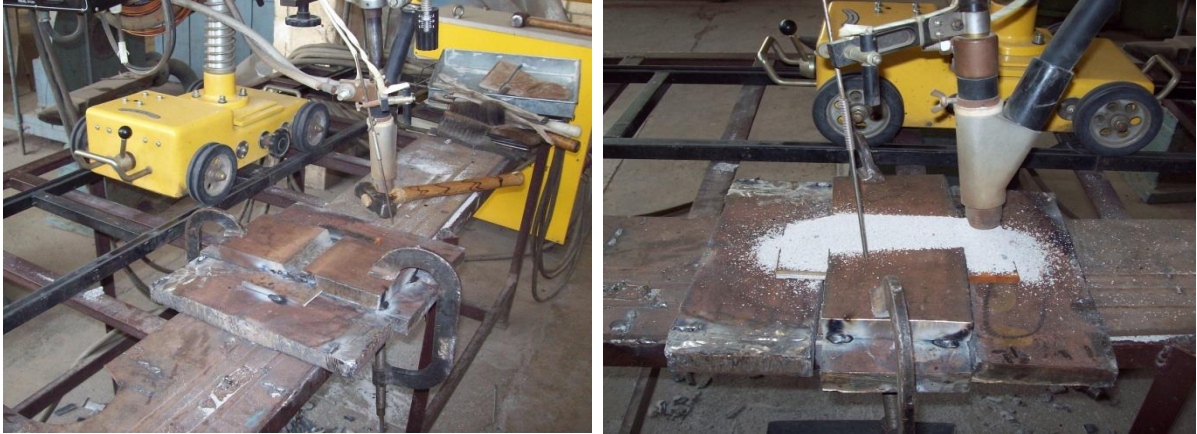
FIGURE 3.12- Submerged arc welding of plates
