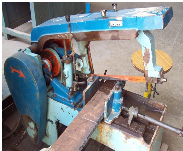
FIGURE 3.5 -Cutting of steel strip through power hacksaw (Courtesy: Central Workshop, Thapar University, Patiala)
