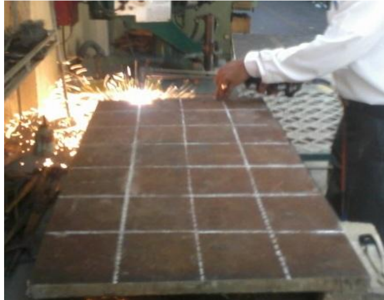
FIGURE 3.4 -Cutting of steel plates through oxy-acetylene gas cutting
