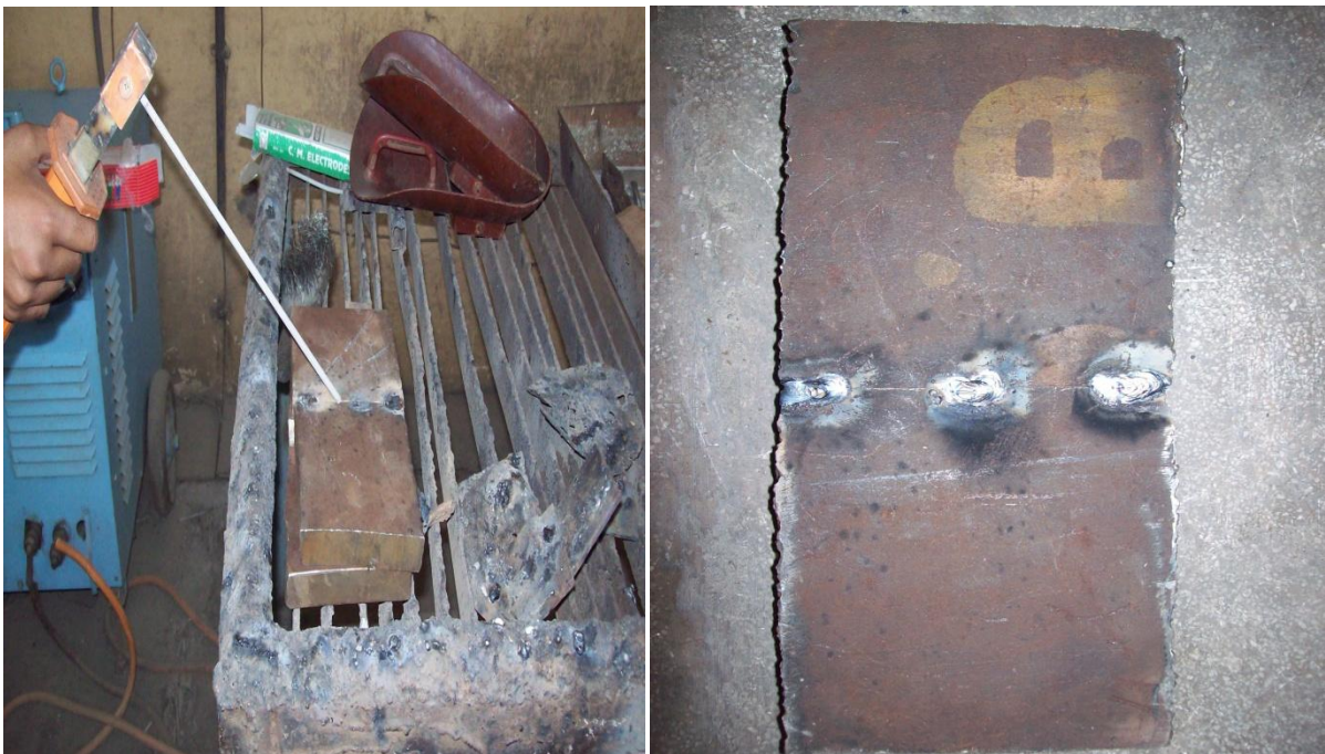
FIGURE 3.9- Tacking on back side of plates
